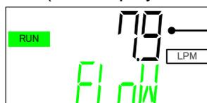
Circulating fluid flow The display flow rate does not include the circulating fluid flow rate flowing in the bypass of this product.
