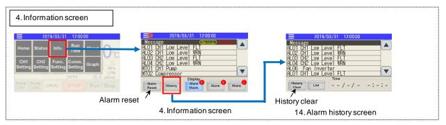
Fig.5-2 Flow chart of operation screen (1/3)
