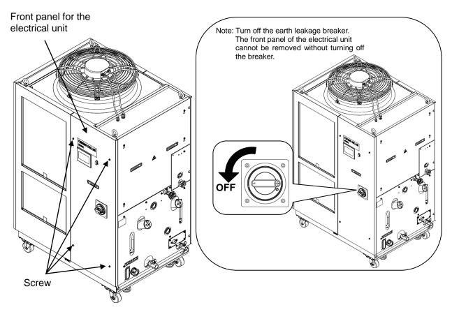
Fig. 3-6 Remove the front panel for the electrical unit
