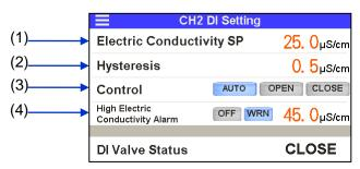
Electric conductivity and alarm (AL27) setting
