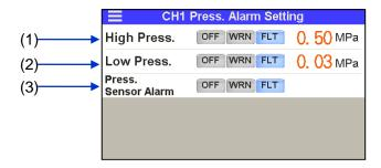
Setting of discharge pressure alarm (AL18/AL19/AL20)
