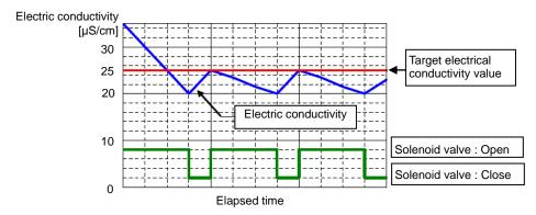
Fig.5-7 Example of electrical conductivity control
