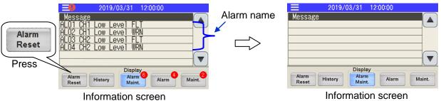
2. Touch the "Alarm" or "Maintenance reminder" on the "Information" screen to display details of the alarm. Touching alarm one time displays the alarm information. Touching alarm twice displays alarm information details. If the alarm utilizes a sub-code, this is displayed in the alarm information details.
