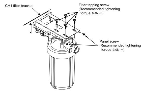
Fig. 3-17 CH1 side Installation of filter bracket.
