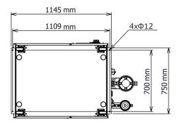
Dimensions for the positions of the anchor bolts (View A)
