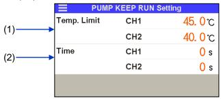
Setting for continuous pump operation
