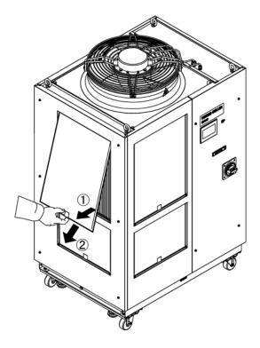
Fig. 7-1 Removal of the dust-proof filter
