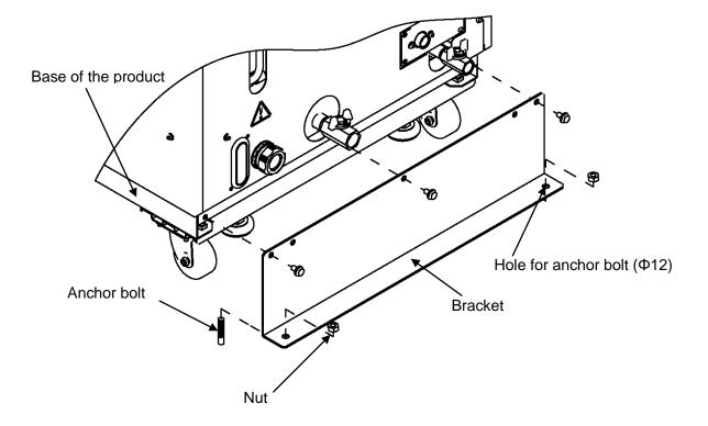
Fig. 3-4 Installation procedures
