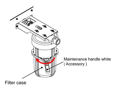
Fig. 3-21 CH1 particle filter case removal
