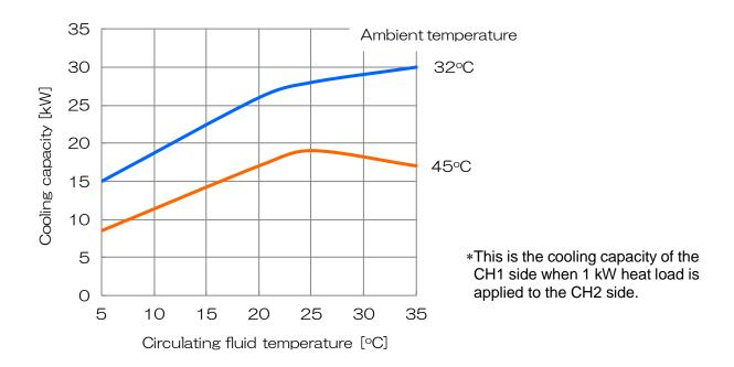
Fig. 8-7 Cooling Capacity (HRL300-A\*-20)
