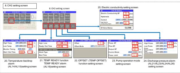
Fig.5-3 Flow chart of operation screen (2/3)
