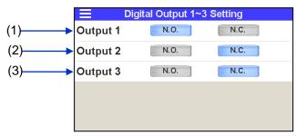
Setting of contact output signal 1 to 3
