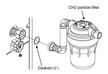
Fig. 3-19 CH2 side Installation of particle filter
