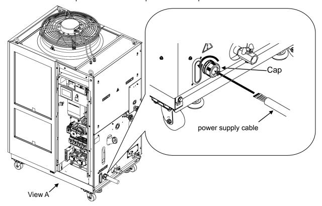
Fig. 3-8 Wiring of power supply cable
