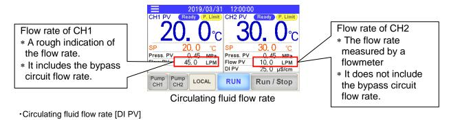
**8.** Display the electric conductivity of CH1,CH2. In the case of option D1 "CH1 with electrical conductivity control", it will display.
