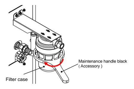
Fig. 3-22 CH2 particle filter case removal
