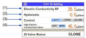
Electric conductivity and alarm (AL28) setting
