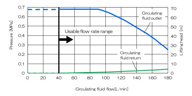
Fig. 8-11 Pump capacity(HRL300-A\*-20 CH1)
