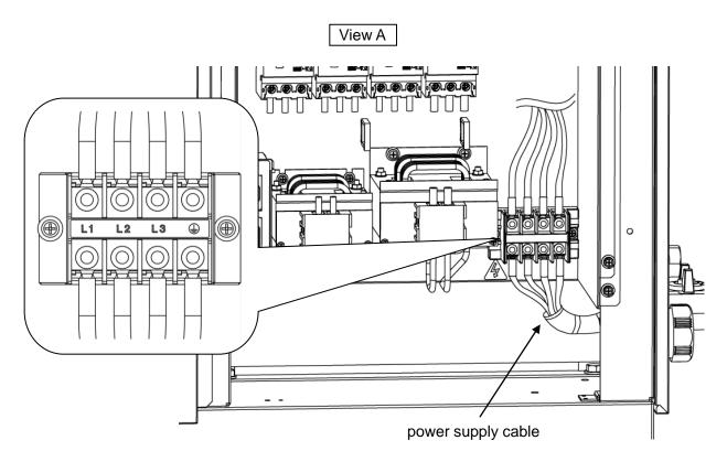
Fig. 3-9 Wiring of power supply cable
