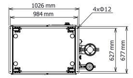
Dimensions for the positions of the anchor bolts (View A)
