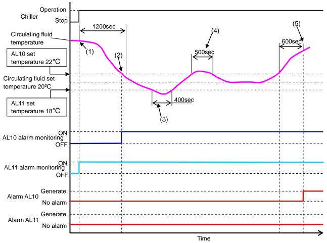
Fig. 5-5 Alarm monitoring timing
