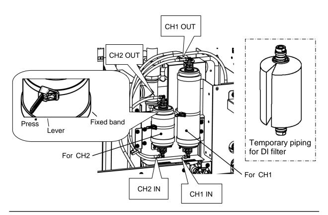
**4.** Pull out the DI filter to the front. The DI filter has been connected to the tube. Please allow excessive force is not applied to the tube. (\*Same for CH1 side)
