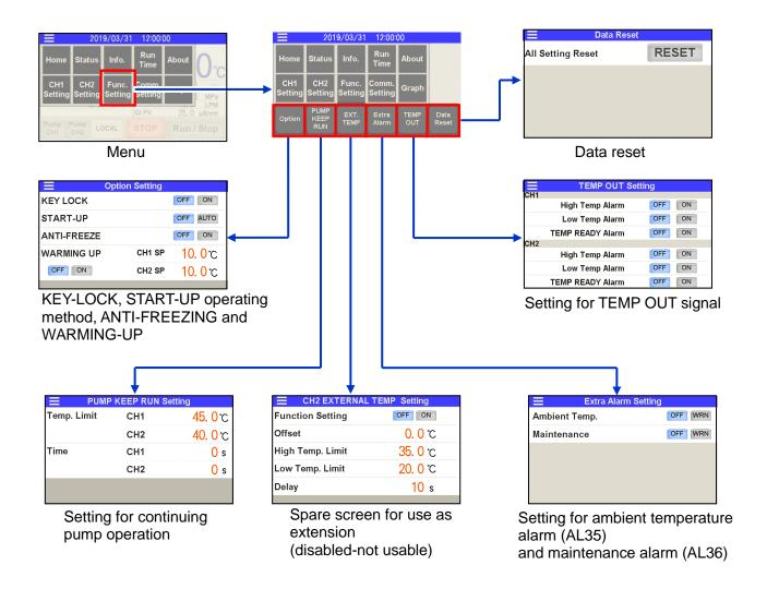
·KEY-LOCK, START-UP operating method, ANTI-FREEZING and WARMING-UP
