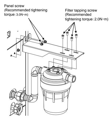
Fig. 3-20 CH2 side Installation of filter bracket.
