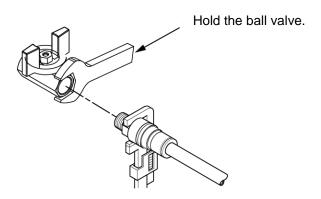
Fig. 3-24 Connection to the drain port
