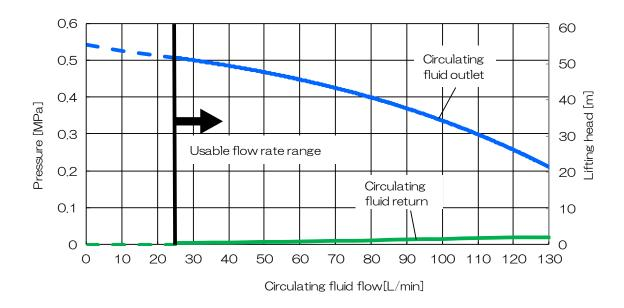
Fig. 8-10 Pump capacity(HRL200-A\*-20 CH1)
