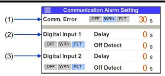
Communication error, detection of contact input signal and operation setting
