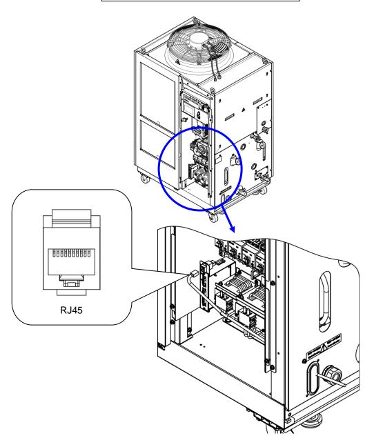
Fig. 3-14 Ethernet Modbus/TCP communication wiring
