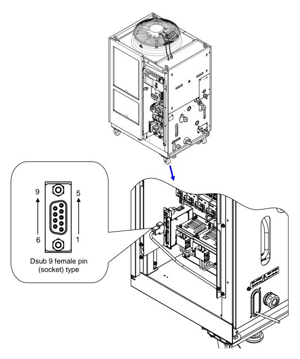
Fig. 3-12 RS-485 communication wiring
