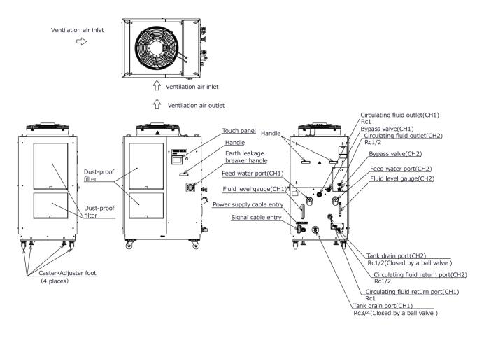
Fig. 2-2 Names of the parts (This drawing shows "HRL200-A-20".)
