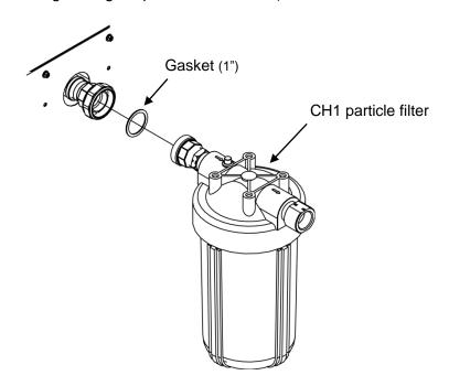
Fig. 3-16 CH1 side Installation of particle filter
