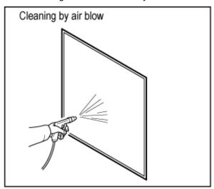
Fig. 7-2 Cleaning of the dust-proof filter
