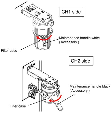
Fig. 7-3 Particle filter removal
