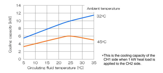
Fig. 8-5 Cooling Capacity (HRL100-A\*-20)
