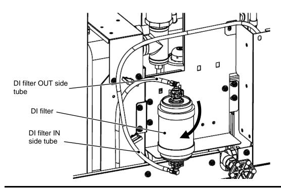
**5.** The connection fitting of the DI filter and the tube is connected by a fastener. O ring is used for the connection fitting. After removing the fastener, remove the connection fitting. Be careful not to apply force to the tube at this time. Also, please be careful not to damage the Oring.
