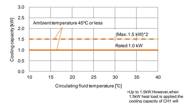
Fig. 8-8 Cooling Capacity (HRL100/200/300-A\*-20)
