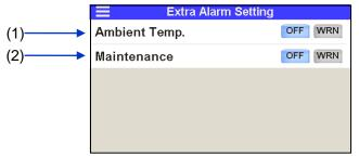
Setting for ambient temperature alarm (AL35) and maintenance alarm (AL36)
