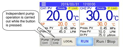
Fig.4-5 Pump independent operation
