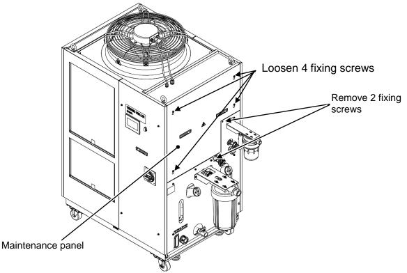
Fig. 7-5 Maintenance panel removal
