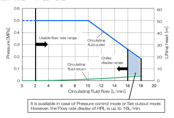
Fig. 8-12 Pump capacity(HRL100/200/300-A\*-20- CH2)
