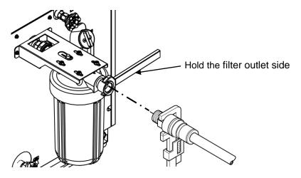
Fig. 3-23 Hold the filter outlet side
