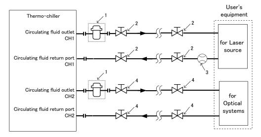
Fig. 3-25 Recommended piping circuit
