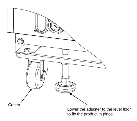
Fig. 3-5 Installation by adjuster foot
