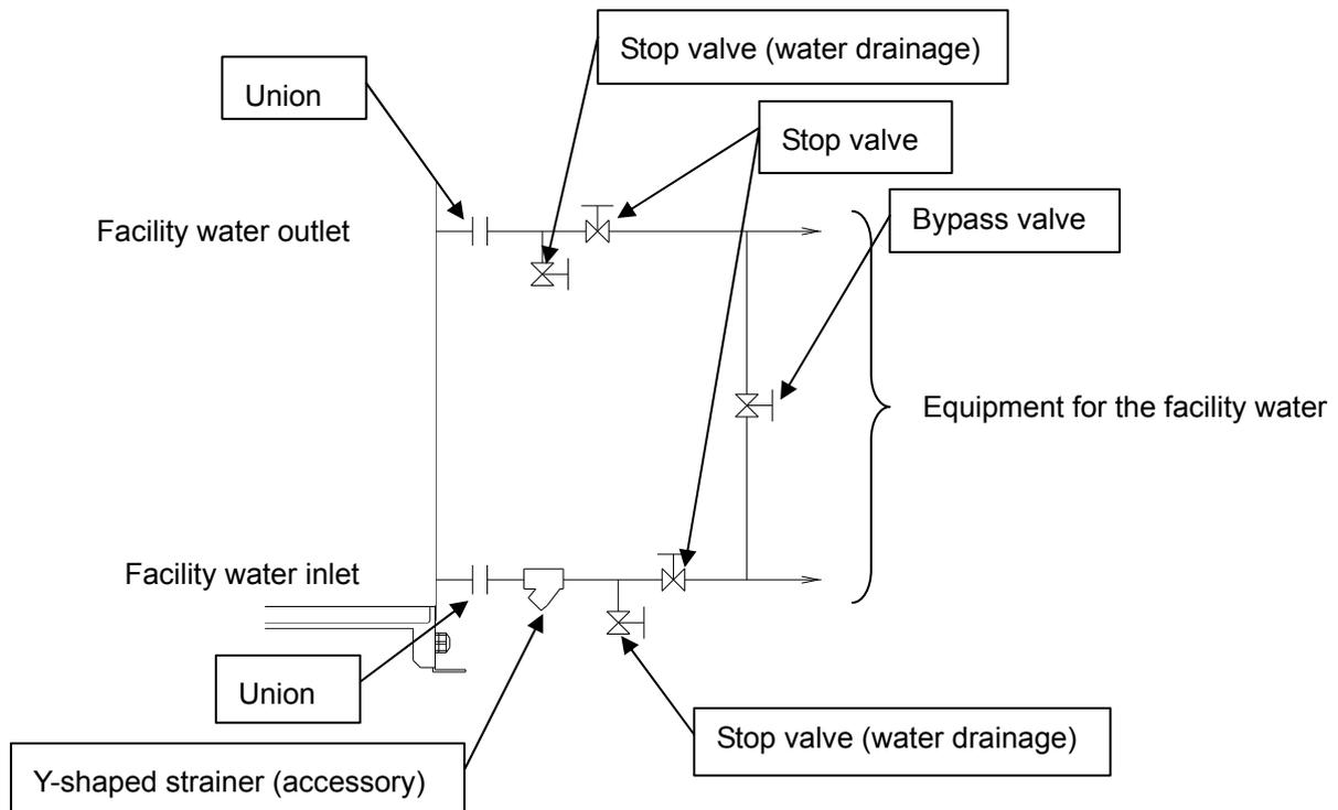
This equipment and facility water piping should be easy to disassemble so that the water-cooled condenser can be cleaned.
