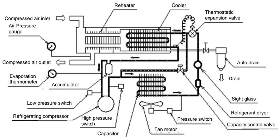
**IDF240D Compressed Air and refrigerant circuits**
