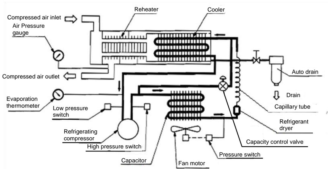
**IDF190D Compressed Air and refrigerant circuits**
