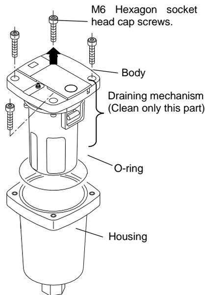
Fig. 2 Disassembly
