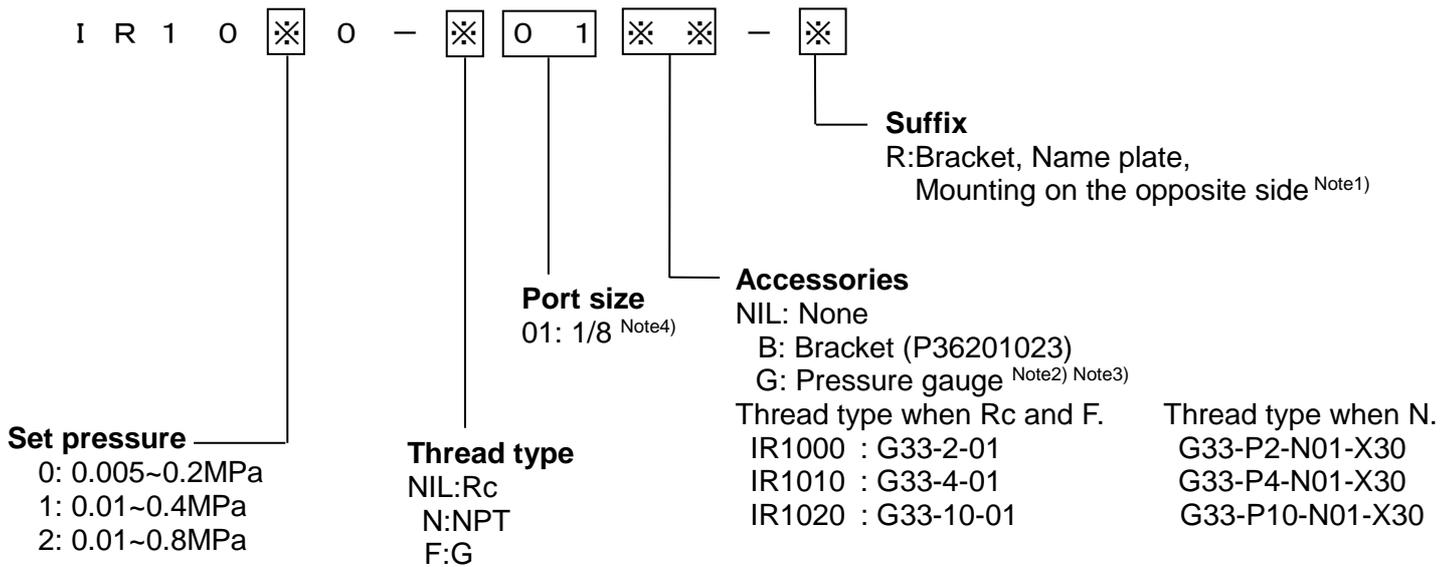
(Note 1) In the standard mounting position, the product name plate is attached to the front and the bracket is mounted to the back when viewed with the SUP side on the left and OUT side on the right.
