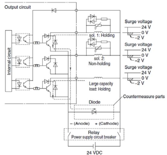
Figure 2. Surge intrusion countermeasure example (NPN outlet example)
