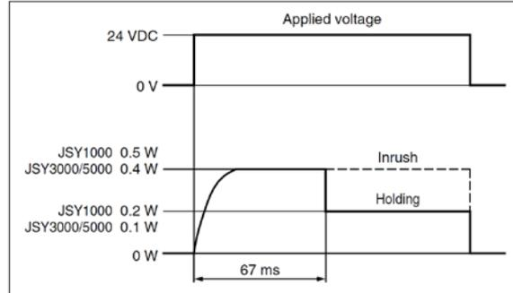
Since the voltage will drop by approx. 0.5 V due to the transistor, pay attention to the allowable voltage fluctuation. (For details, refer to the solenoid specifications of each type of valve.)
