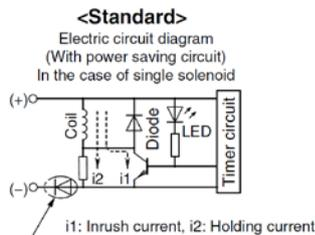
The circuit shown to the left reduces the power consumption for holding in order to save energy. Refer to the electrical power waveform as shown below.
