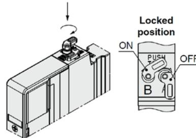
Carefully check the manual override projection amount. Max. (at OFF): 3.7 mm
