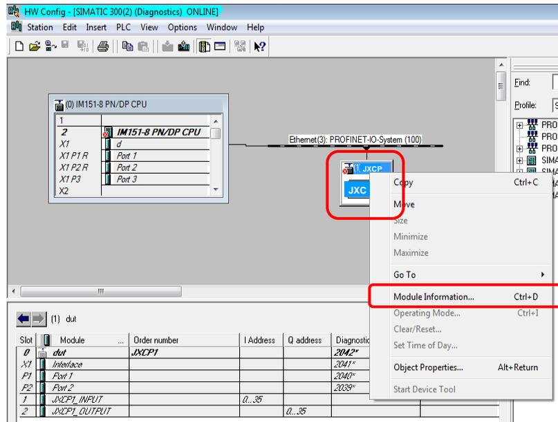
Fig.15.1 Selection of [Module Information] of HW Config
