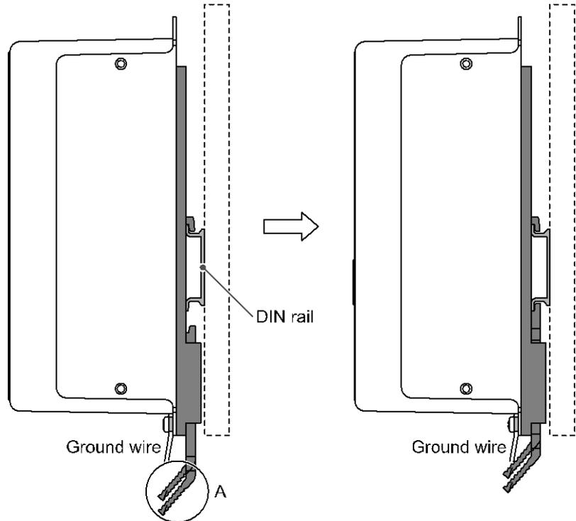
Hook the controller on the DIN rail and press lever A in the direction of the arrow to lock it.
