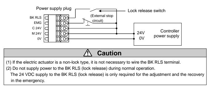
After the wiring of the power supply plug is completed, connect it to the CN1 connector of the controller. Please refer to **"5.3 Wiring of power supply plug"** for how to wire the power supply plug.
