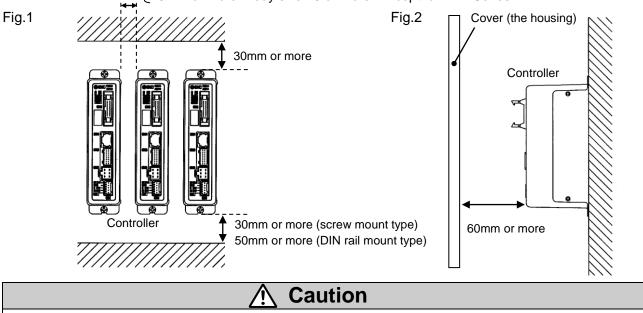
If the mounting surface of the controller is distorted or not flat, excessive force may be applied to the housing, etc. causing malfunction.
