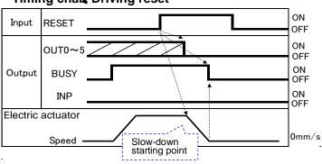
If the electric actuator is within the "In position" range, INP will be turned ON.
