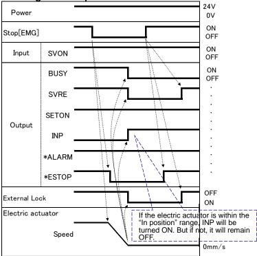
The "\*ALARM" and "\*ESTOP" are expressed as negative-logic circuit. When "Stop" is OFF, the stop is activated.
