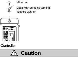
The M4 screw, cable with crimping terminal, and toothed washer should be obtained separately.
