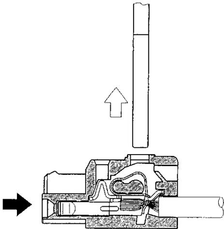
4) Releasing the screwdriver connects the cable.
