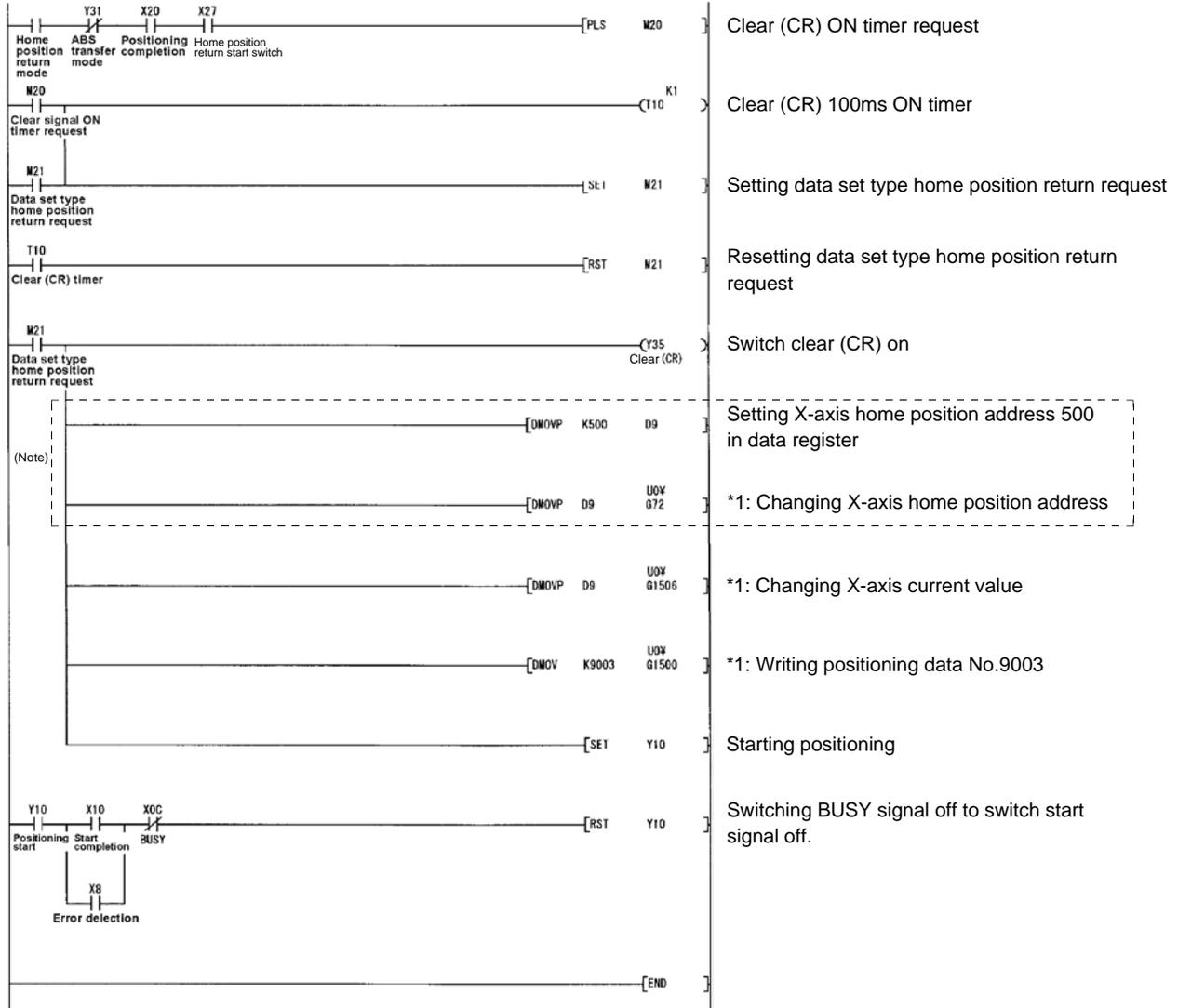
Note. When the data of the home position address parameter is not written from GX Developer or the like before starting the data set type home position return program, this sequence circuit is required.
