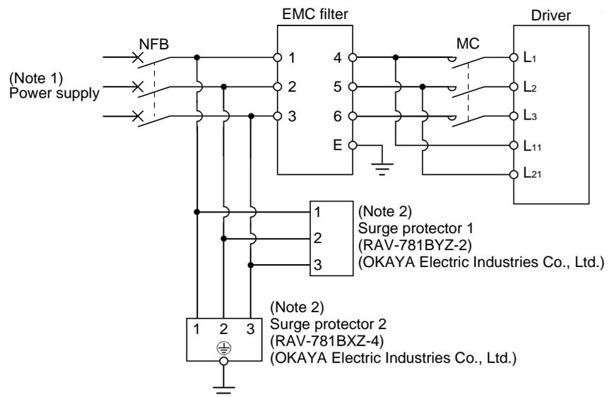
Note 1. For 1-phase 200 to 230VAC power supply, connect the power supply to L<sub>1</sub>, L<sub>2</sub> and leave L<sub>3</sub> open.
