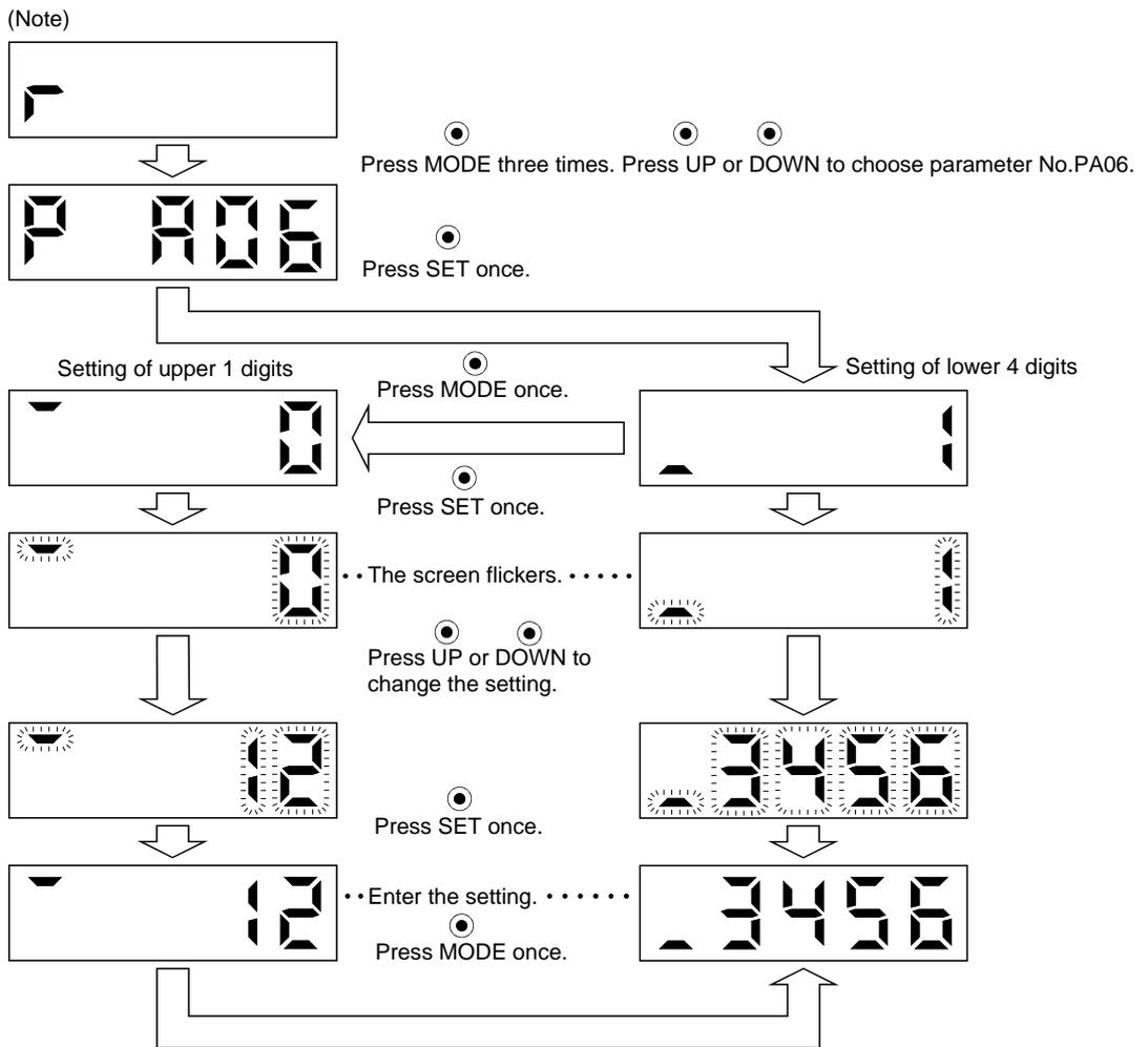
Note. The example assumes that the status display screen that appears at power-on has been set to the servo motor speed in parameter No.PC36.
