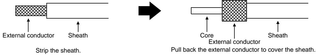
(1) For CN1 connector (Sumitomo 3M Limited connector)
