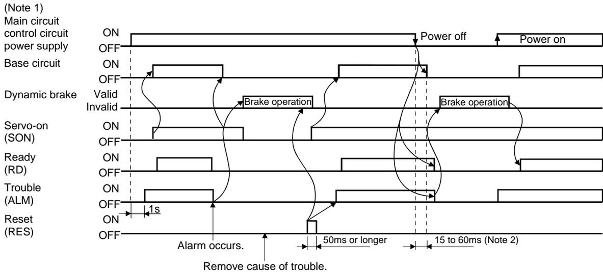
Note 1. Shut off the main circuit power as soon as an alarm occurs.
