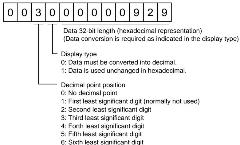
Since the display type is "0" in this case, the hexadecimal data is converted into decimal.
