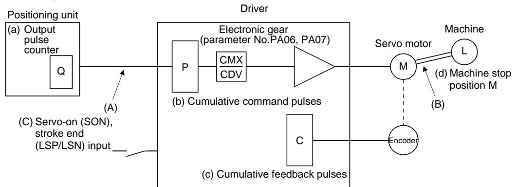
When a position shift occurs, check (a) output pulse counter, (b) cumulative command pulse display, (c) cumulative feedback pulse display, and (d) machine stop position in the above diagram.
