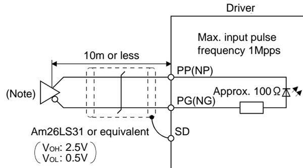
Note. Pulse train input interface is comprised of a photo coupler.
