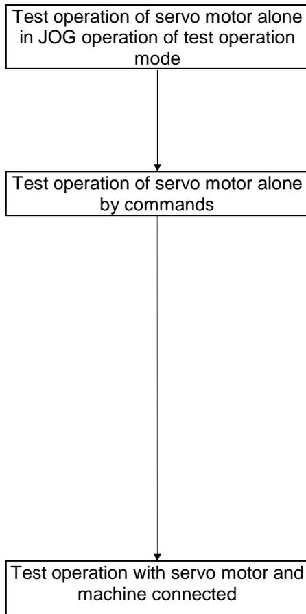
In this step, confirm that the driver and servo motor operate normally.
