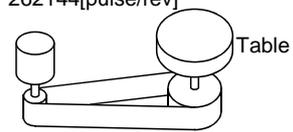
$$\frac{CMX}{CDV} = \Delta \theta^\circ \cdot \frac{Pt}{\Delta \theta} = 0.01 \cdot \frac{262144}{625/12544 \cdot 360} = \frac{102760448}{703125} \dots \dots \dots (5.1)$$
