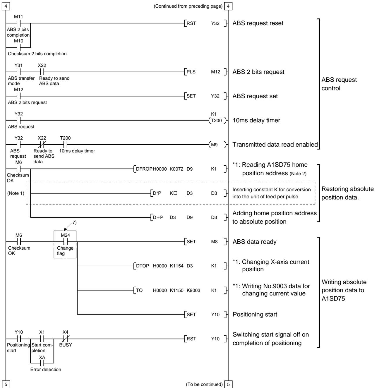
Note 1. When the unit setting parameter value of the A1SD75 positioning module is changed from "3" (pulse) to "0" (mm), the unit is  $\times 0.1\mu\text{m}$  for the input value. To set the unit to  $\times 1\mu\text{m}$ , add this program to multiple the feed value by 10.
