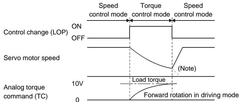
Note. When the start (ST1 · ST2) is switched off as soon as the mode is changed to speed control, the servo motor comes to a stop according to the deceleration time constant.
