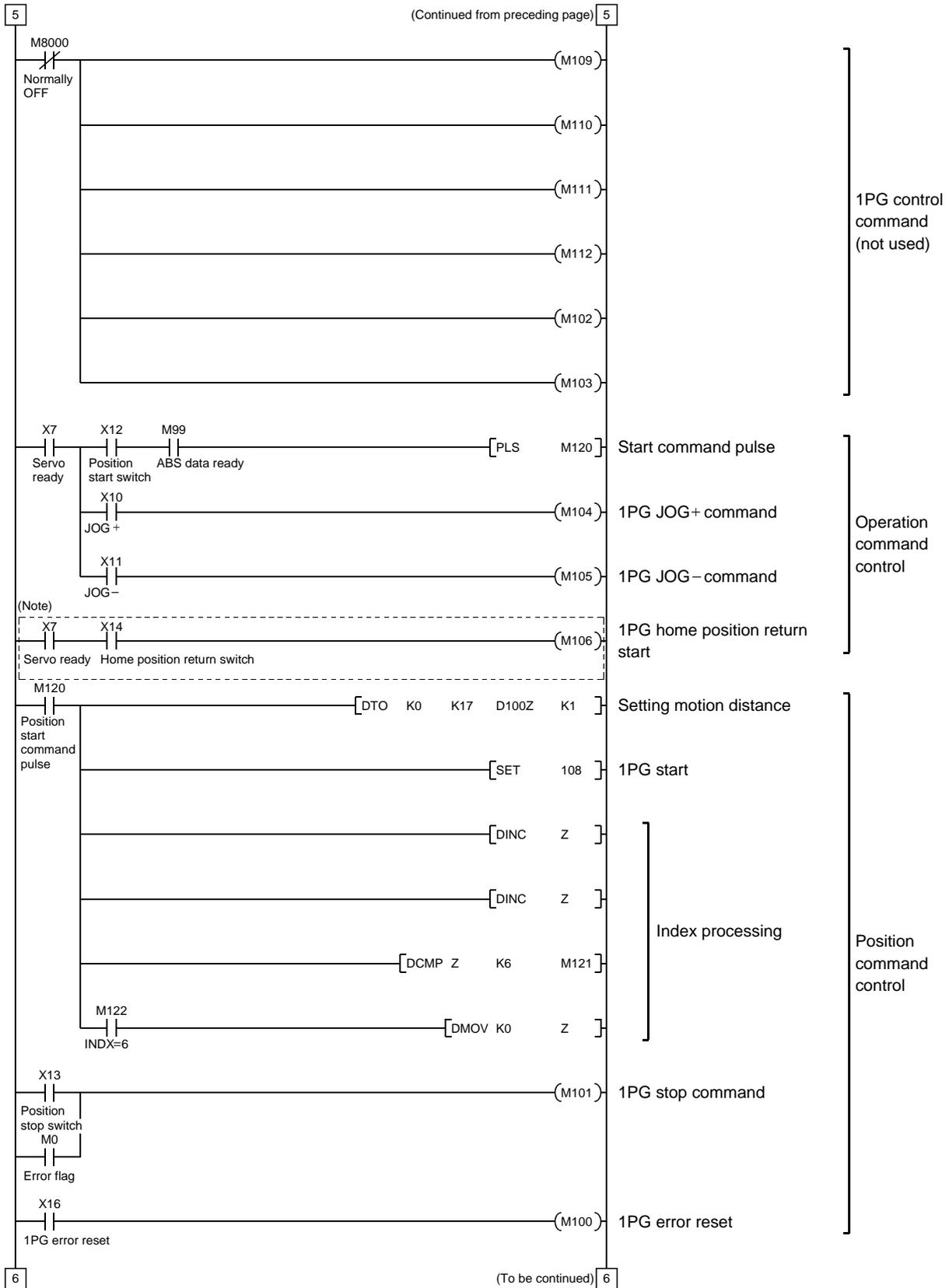
Note. Program example for the dog type home position return. For the data set type home position return, refer to the program example in (2), (d) of this section.
