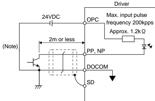
Note. Pulse train input interface is comprised of a photo coupler.
