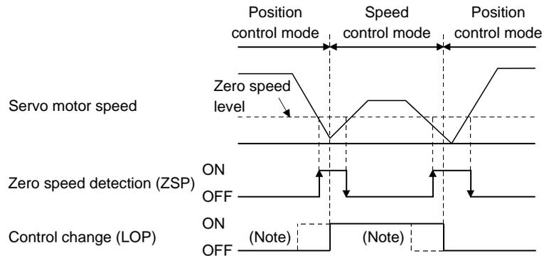
Note. When ZSP is not on, control cannot be changed if LOP is switched on-off. If ZSP switches on after that, control cannot be changed.
