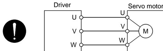
2) The power supplied to the driver should not be connected to the servo motor power supply terminals (U, V, W). To do so will fail the connected driver and servo motor.
