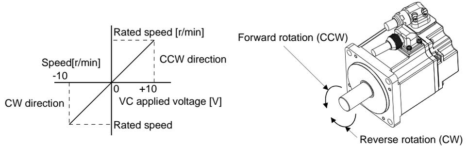
Generated torque limit values will vary about 5% relative to the voltage depending on products. Also the torque may vary if the voltage is low ( $-0.05V$  to  $+0.05V$ ) and the actual speed is close to the limit value. In such a case, increase the speed limit value.
