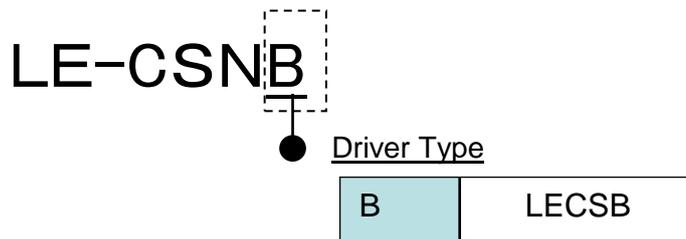
\*LE-CSNB is 10150-3000PE(Connector)/10350-52F0-008 (Shell kit) of Sumitomo 3M Limited or equivalent goods.
