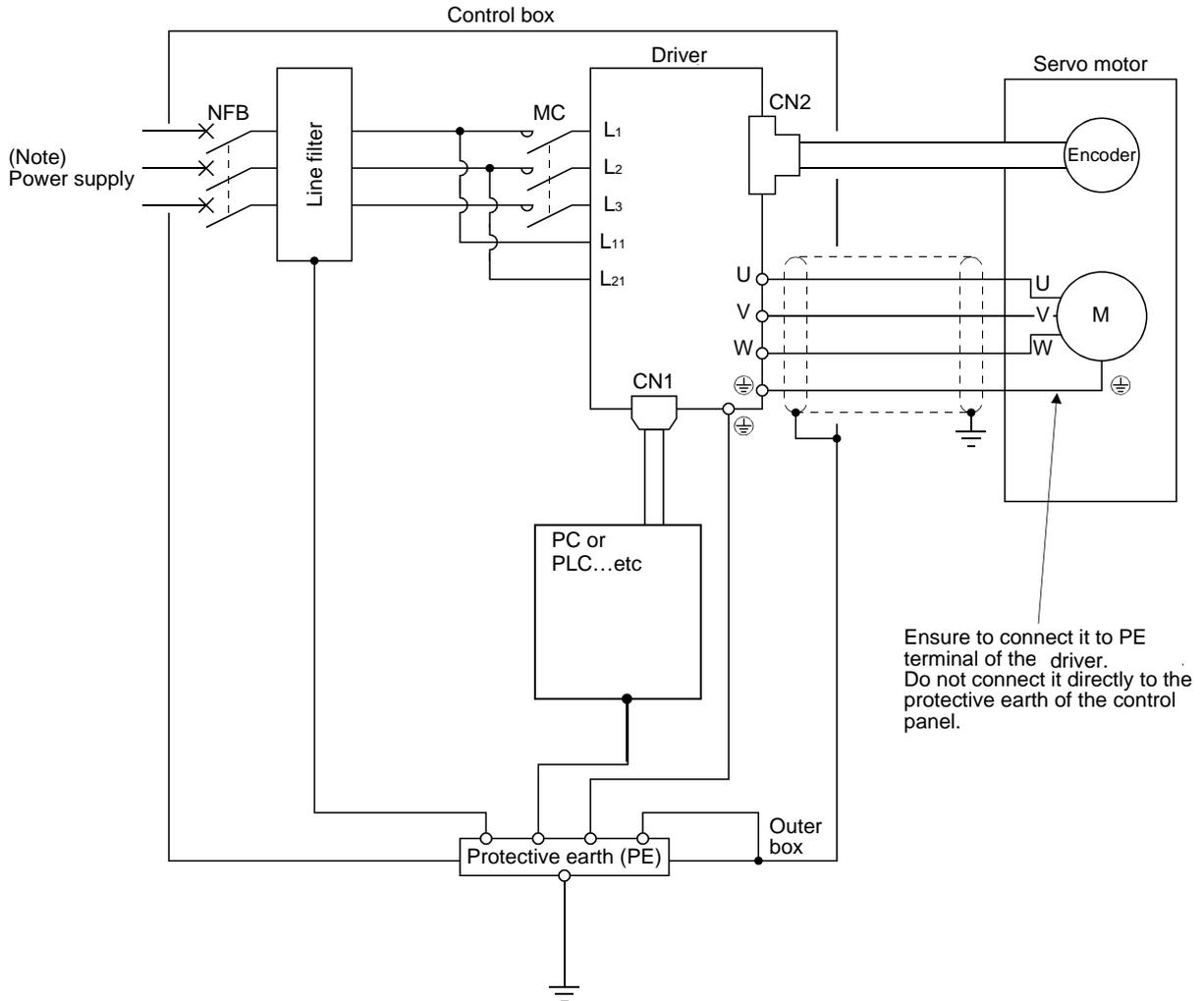
Note. For 1-phase 200 to 230VAC or 1-phase 100 to 120VAC, connect the power supply to L1 \* L2 and leave L3 open.
