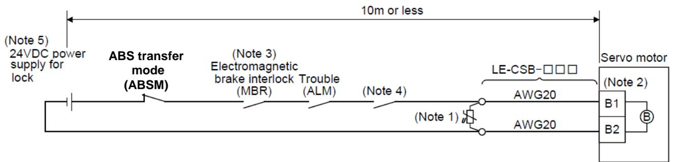
Note 1. Connect a surge absorber as close to the servo motor as possible.
