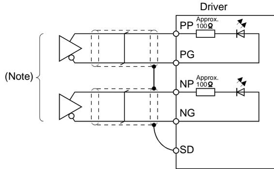
Note. Pulse train input interface is comprised of a photo coupler.
