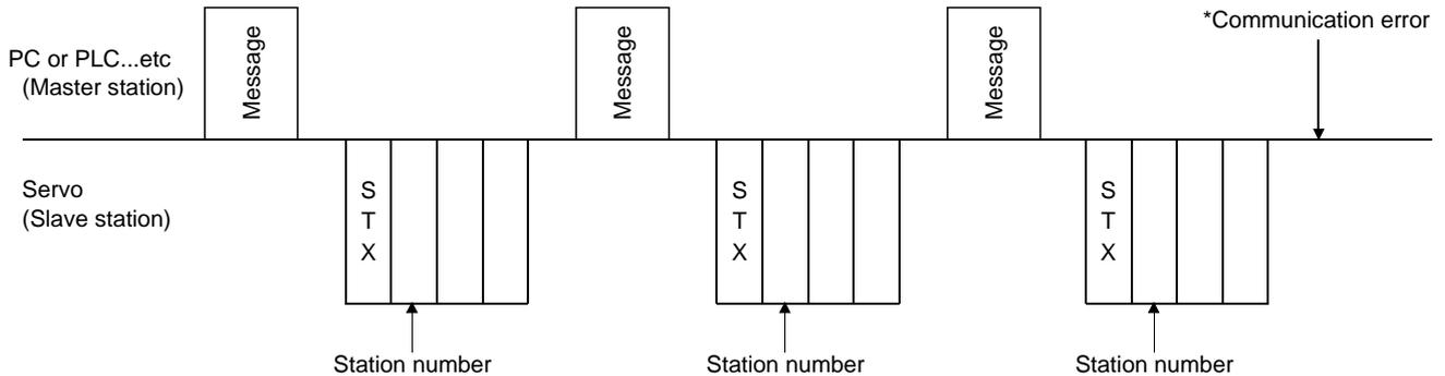
Similarly, when the master station detects a fault (e.g. checksum, parity) in the response data from the slave station, the master station retransmits the message which was sent at the occurrence of the fault. A communication error occurs if the retry processing is performed three times.
