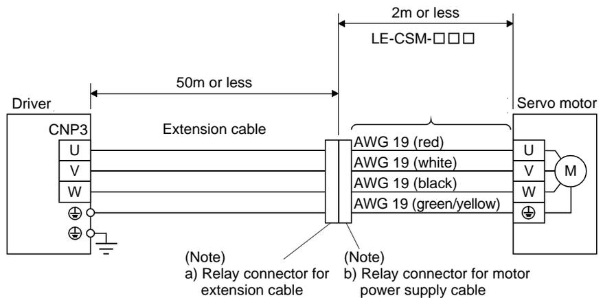
Note. Use of the following connectors is recommended when ingress protection (IP65) is necessary.
