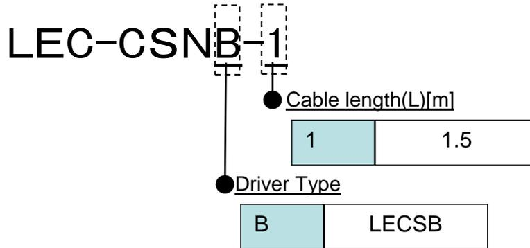
\*LEC-CSNB-1(Connector/ Shell kit) is 10150-3000PE (Connector)/ 10350-52F0-008(Shell kit) of Sumitomo 3M Limited or equivalent goods.
