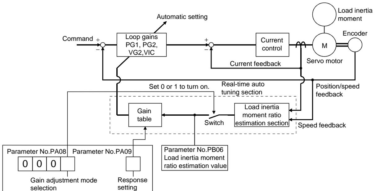
When a servo motor is accelerated/decelerated, the load inertia moment ratio estimation section always estimates the load inertia moment ratio from the current and speed of the servo motor. The results of estimation are written to parameter No.PB06 (the ratio of load inertia moment to servo motor). These results can be confirmed on the status display screen of the software (MR Configurator2™) section.
