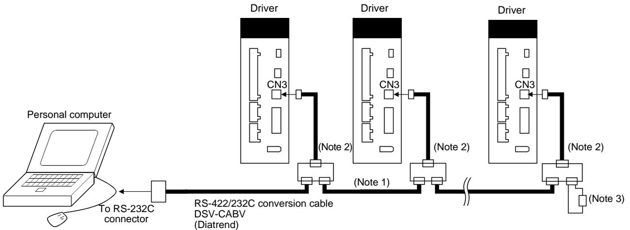
Note 1. Refer to section 13.1 for cable wiring.
