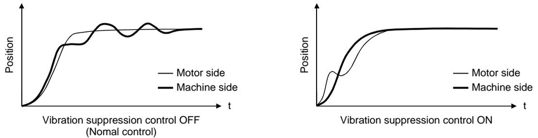
When the advanced vibration suppression control (vibration suppression control tuning mode (parameter No.PB02)) is executed, the vibration frequency at machine side can automatically be estimated to suppress machine side vibration.
