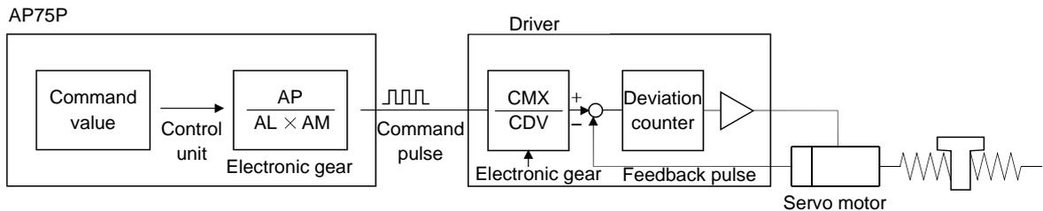
The encoder resolution of the servo motor is 262144 pulses/rev. For example, the pulse command required to rotate the servo motor is as follows.
