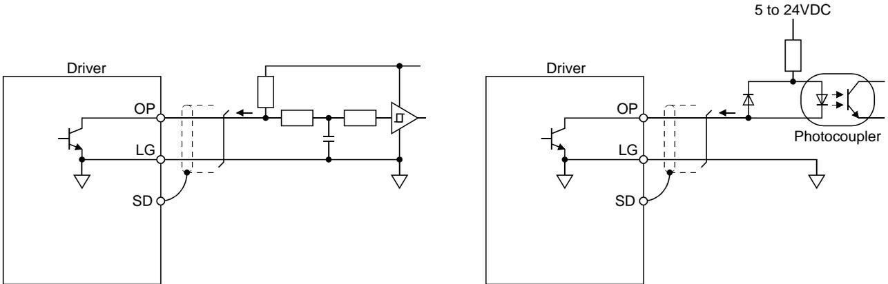
If the encoder Z-phase pulse is open collector method, it supports only to the sink (NPN) type interface. It does not correspond to the source (PNP) type interface.
