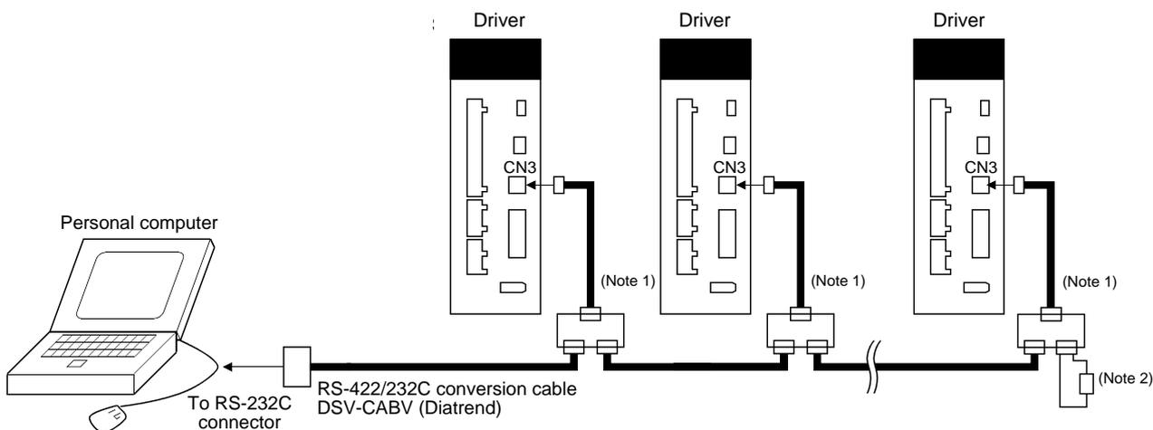
Note 1. The BMJ-8 (Hakko Electric Machine Works) is recommended as the branch connector.
