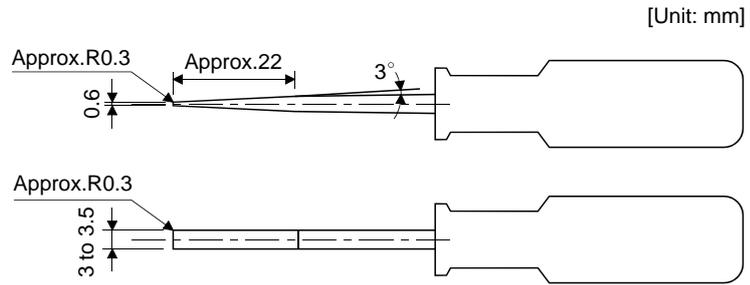
2) When using the flat-blade screwdriver - part 1
