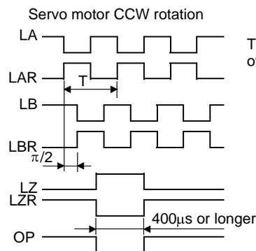
Time cycle (T) is determined by the settings of parameter No. PA15 and PC19.
