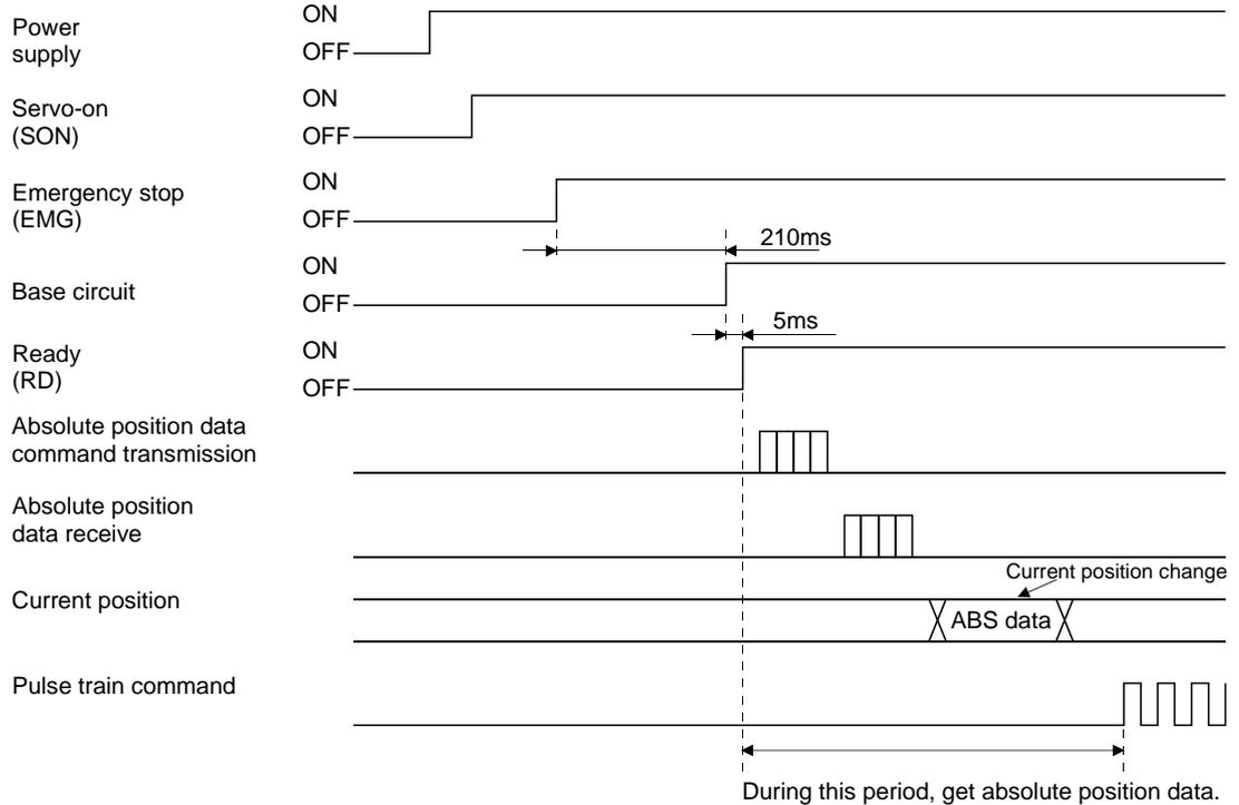
2) When an emergency stop is activated during servo on
