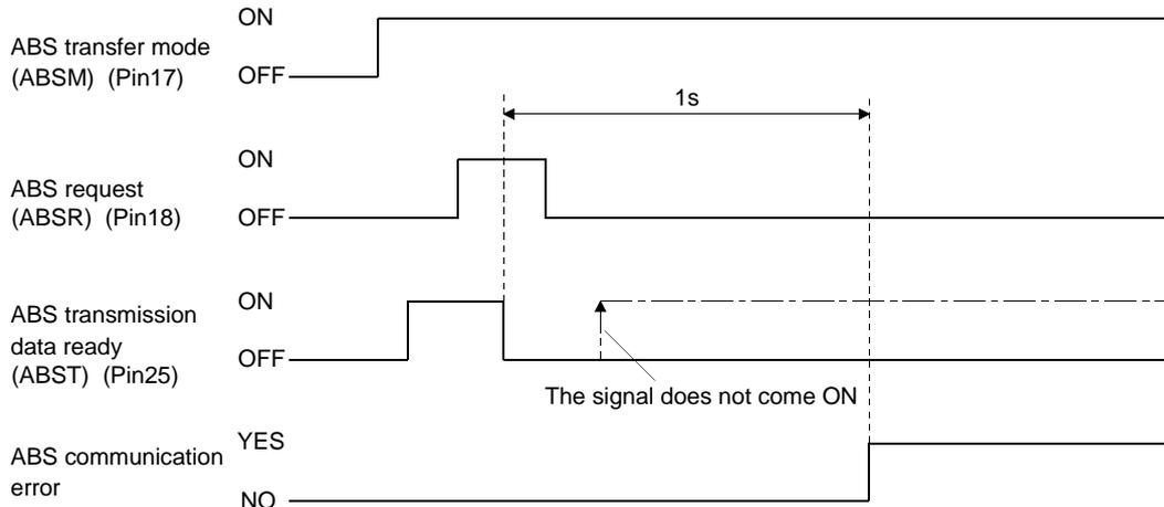
(b) The time required for the ABS transfer mode signal to go OFF after it has been turned ON (ABS transfer time) is checked.
