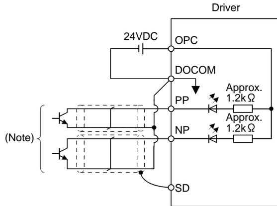
Note. Pulse train input interface is comprised of a photo coupler.
