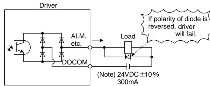
Note. If the voltage drop (maximum of 2.6V) interferes with the relay operation, apply high voltage (up to 26.4V) from external source.
