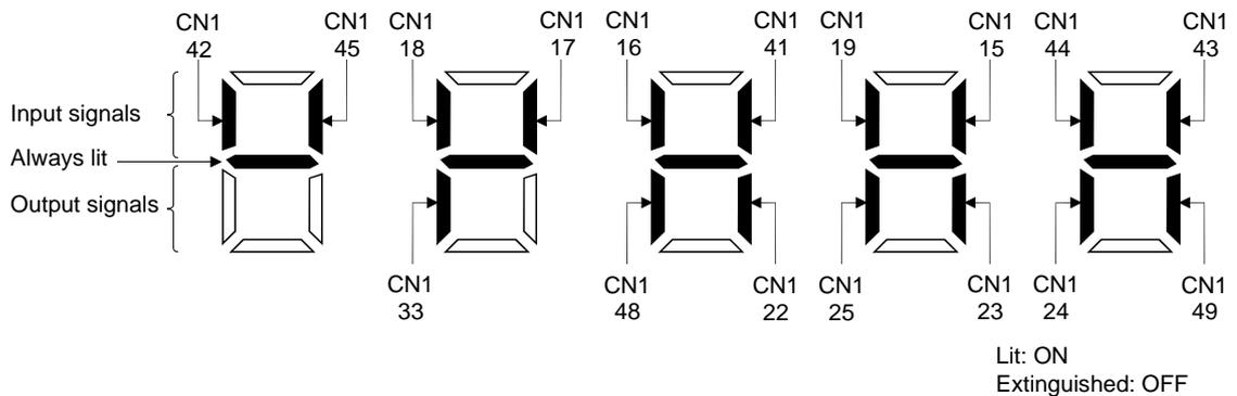
The LED segment corresponding to the pin is lit to indicate ON, and is extinguished to indicate OFF.
