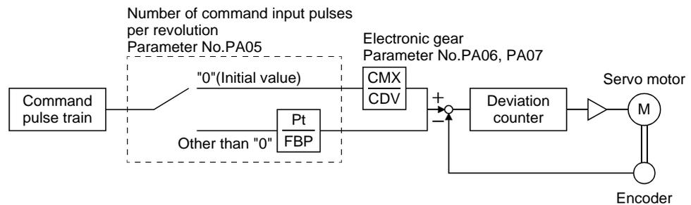
$$\frac{\text{CMX}}{\text{CDV}} = \frac{\text{Parameter No. PA06}}{\text{Parameter No. PA07}}$$
