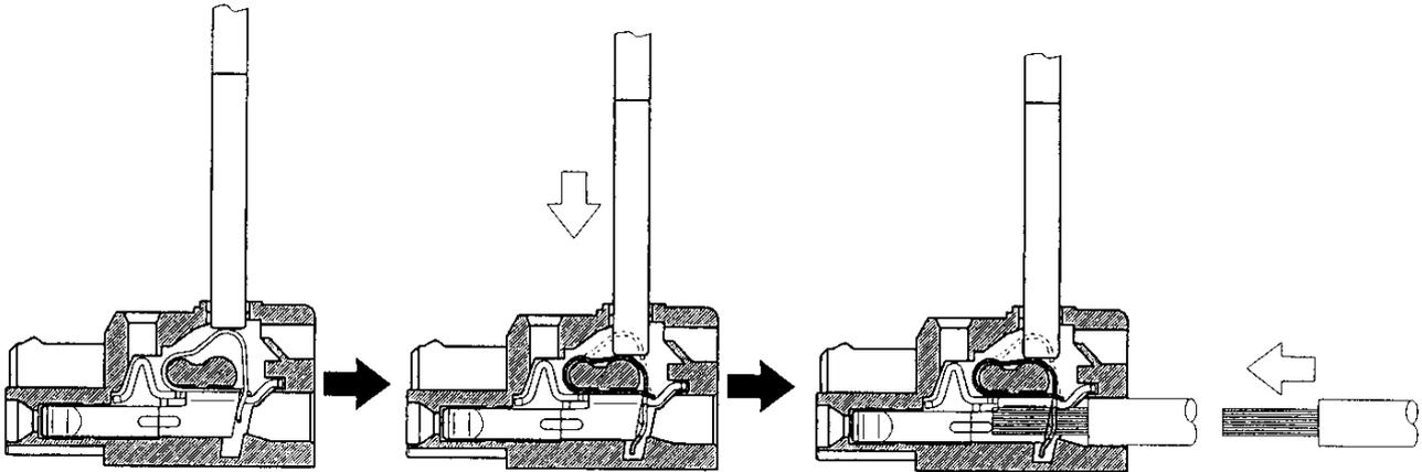
1) Insert the screwdriver into the square window at top of the connector.
