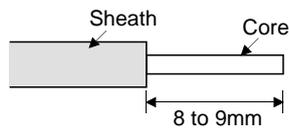
Twisted wire: Use the cable after stripping the sheath and twisting the core. At this time, take care to avoid a short caused by the loose wires of the core and the adjacent pole. Do not solder the core as it may cause a contact fault. Alternatively, a ferrule may be used to put the wires together.
