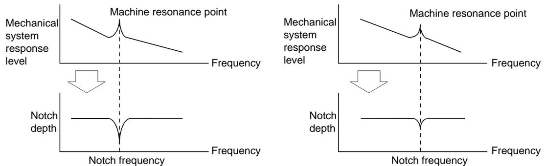
When machine resonance is large and frequency is low
