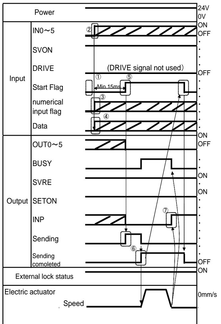
(5) Input the numerical data input flag bit and numerically specified parameter data, and then input RWw1,bit0: Start flag=ON.
