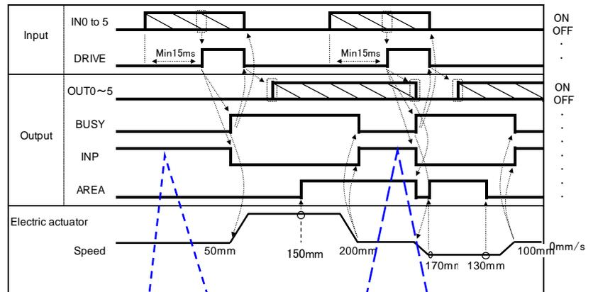
If the now position is inside of step data positioning. The INP signal is ON. Otherwise, the signal is OFF.
