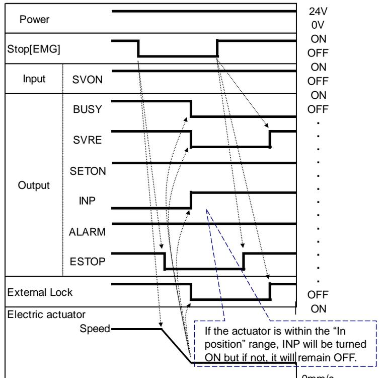
When "Stop [EMG]" is OFF, the stop is activated.
