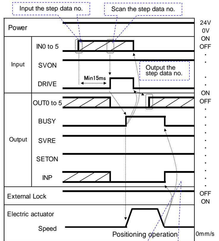
If the electric actuator is within the "In position" range, INP will be turned ON but if not, it will remain OFF.
