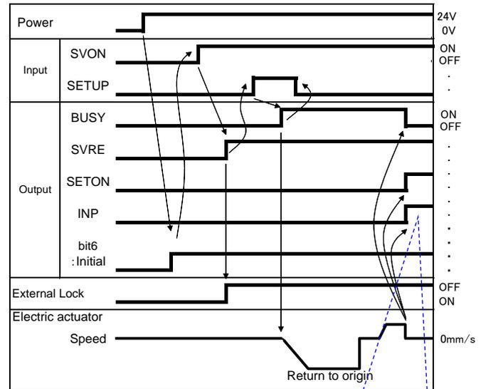
If the electric actuator is within the "In position" range, INP will be turned ON but if not, it will remain OFF.
