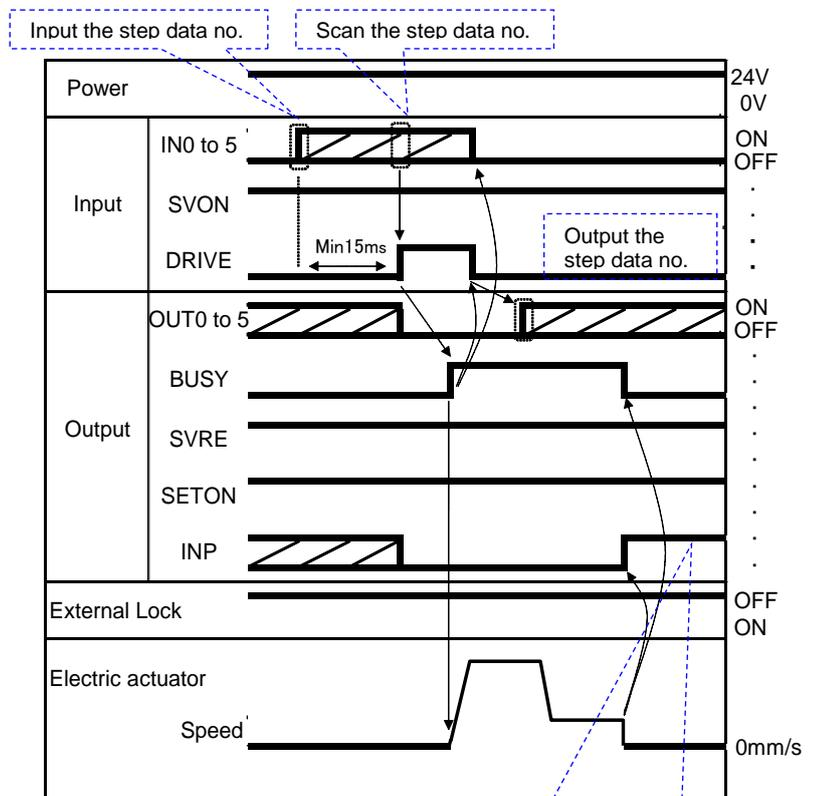
If the electric actuator is within the "In position" range, INP will be turned ON but if not, it will remain OFF.
