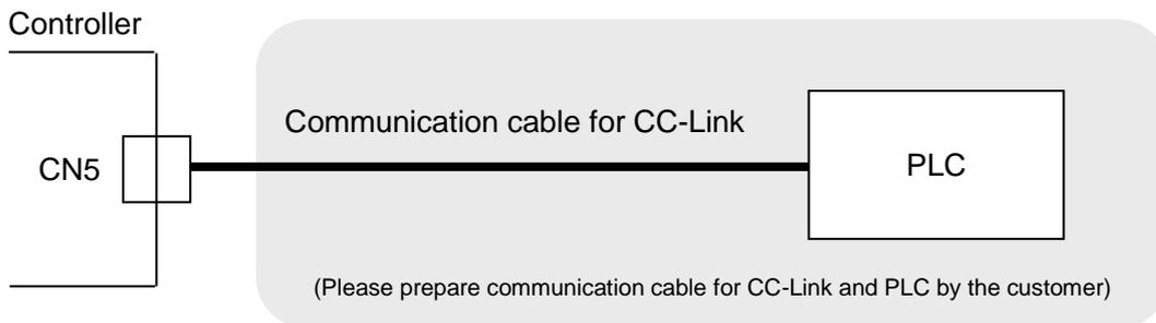
For the wiring method, refer to "7. CN5: Communication Plug Connector".
