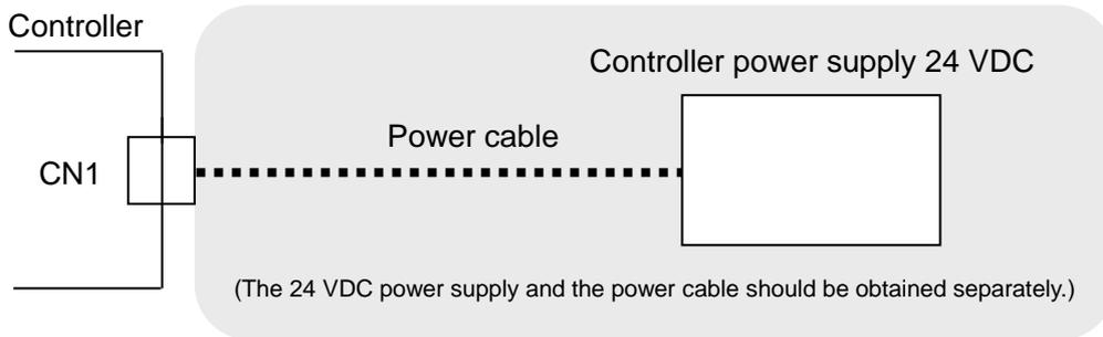
Please refer to “6. CN1: Power supply plug” for how to wire the CN1 connector.
