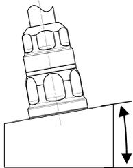
Mount the fitting at an angle to prevent water and detergent from being accumulated in the fitting.
