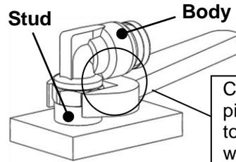
Carefully perform the piping work so that the tool is not in contact with the body.
