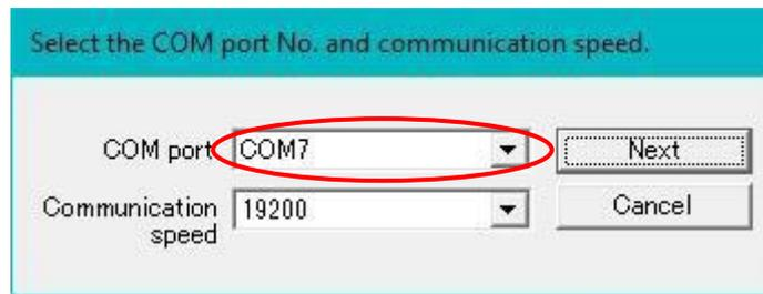
\* If "COM port Not Available" is displayed and/or the number of COM port to which a controller setting cable is connected is not displayed as shown above, the controller setting cable is not recognised. Confirm that the wiring and two drivers are properly installed (Refer to "3. Check of the Communication Port").
