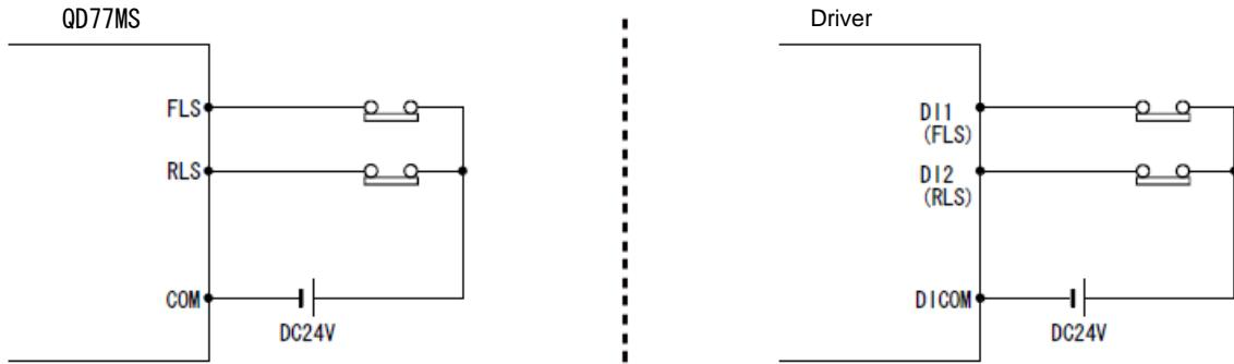
Note) The upper limit switch should be installed in the direction in which the "Current feed value" increases. The lower limit switch should be installed in the direction in which the "Current feed value" decreases.
