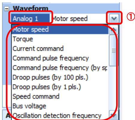
The analogue and digital waveforms that can be set with LECSS2-T are shown below.
