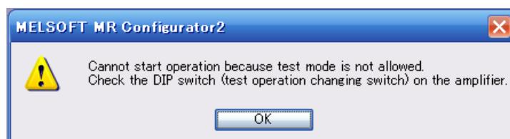
When performing the test operation mode using the set-up software (MR Configurator2<sup>TM</sup>), set the test operation select switch to the “UP” position.
