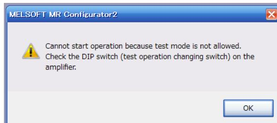
When performing the test operation mode using the set-up software (MR Configurator2™), set the test operation select switch to the "UP" position.
