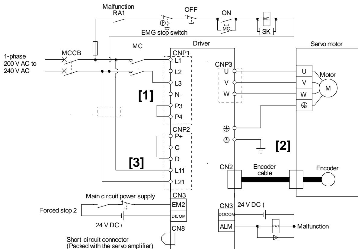
[1] Power supply input terminals, L<sub>1</sub>, L<sub>3</sub>: Provide specified power supply to input terminals L<sub>1</sub> and L<sub>2</sub>.
