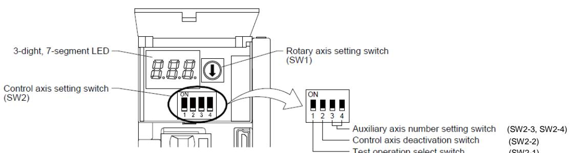
For the test operation select switch(SW2-1), please refer to section 4 of LECSS2-T Operation Manual (Simplified edition).
