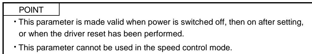
Set this parameter when using the absolute position detection system in the position control mode.
