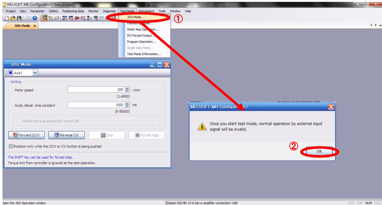
In the test operation mode, if the test operation select switch (SW2-1) is in the “Down” position, the following warning is displayed.
