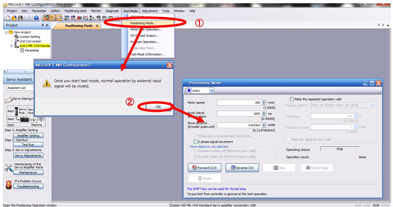
In the test operation mode, if the test operation select switch (SW2-1) is in the "Down" position, the following warning is displayed.
