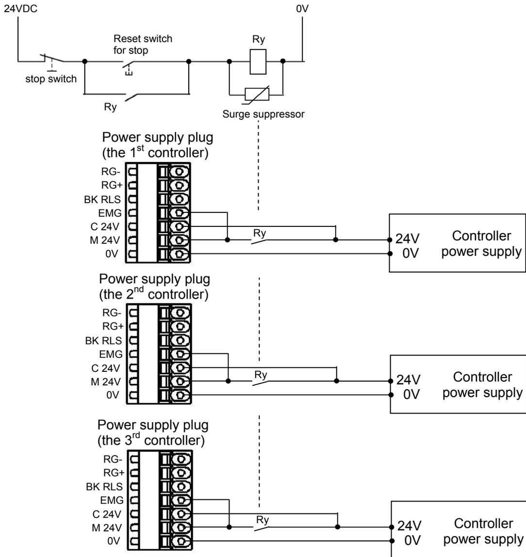
The relay must be a safety relay or monitored by a safety relay.
