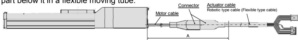
9. **The cable connecting the actuator and controller is superior in bending resistance, but should not be placed into a flexible moving tube with a radius smaller than the specified value.**
