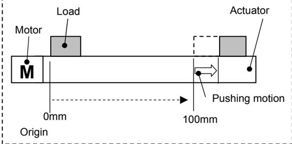
Step No.2 Positioning operation (Example)
