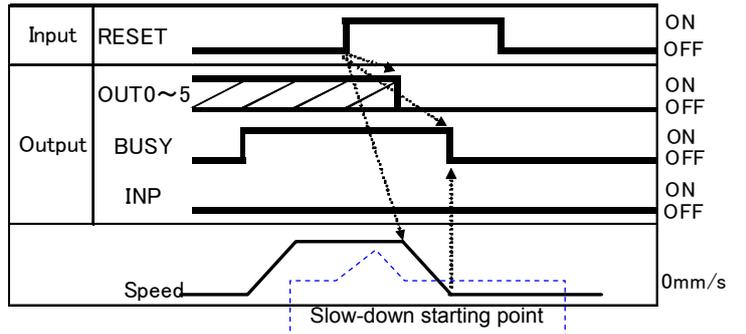
\* If the actuator is within the "In position" range, INP will be turned ON.
