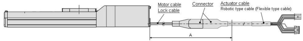
9. **Select "Robotic type cables" in case of inflecting actuator-cable repeatedly. And do not put cables into a flexible moving tube with a radius smaller than the specified value. (Min. 50mm).**
