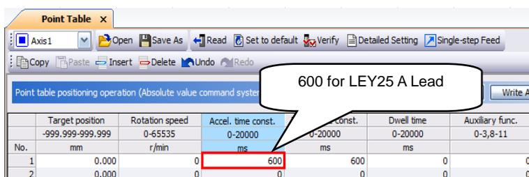
\*5. Use the acceleration time constant of Point table No.1 as the acceleration time constant (msec) of Home position return. Set the recommended value in the above figure. Refer to "LECSB2-T□ Operation Manual (Simplified Edition)", section 5.7 for how to set the Point table.
