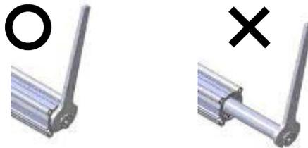
11. When rotational torque is applied to the plate end, use within the allowable range. [LEYG series]
