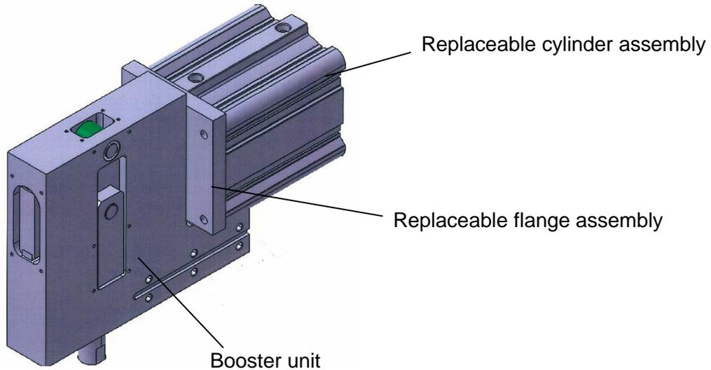
Refer to the replacement procedure for the replacement of the cylinder.
