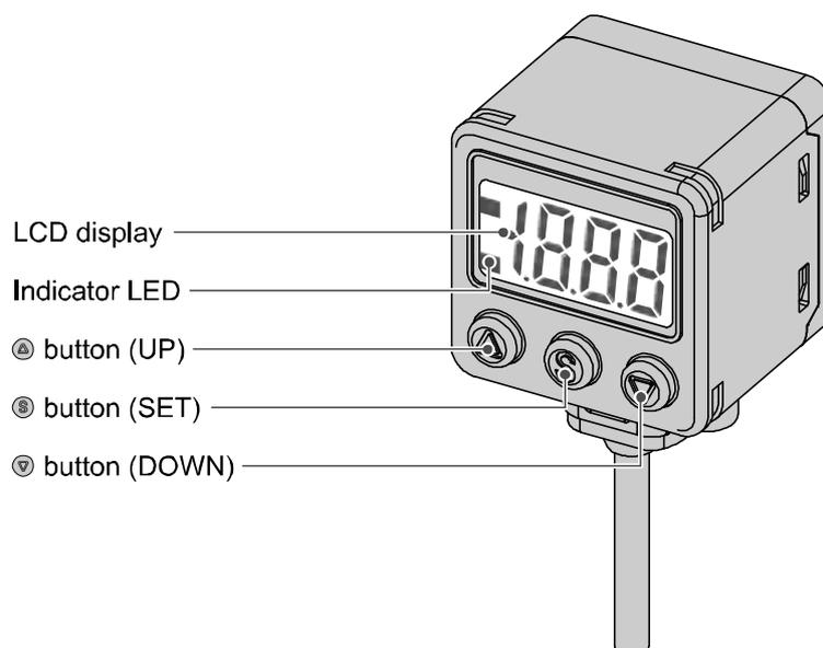
Indicator LED (Orange LED): Displays the switch output condition.
