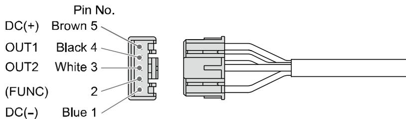
Internal circuit and wiring example
