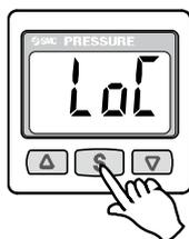
Press the **Δ** and **▽** buttons simultaneously for 5 seconds or longer.
