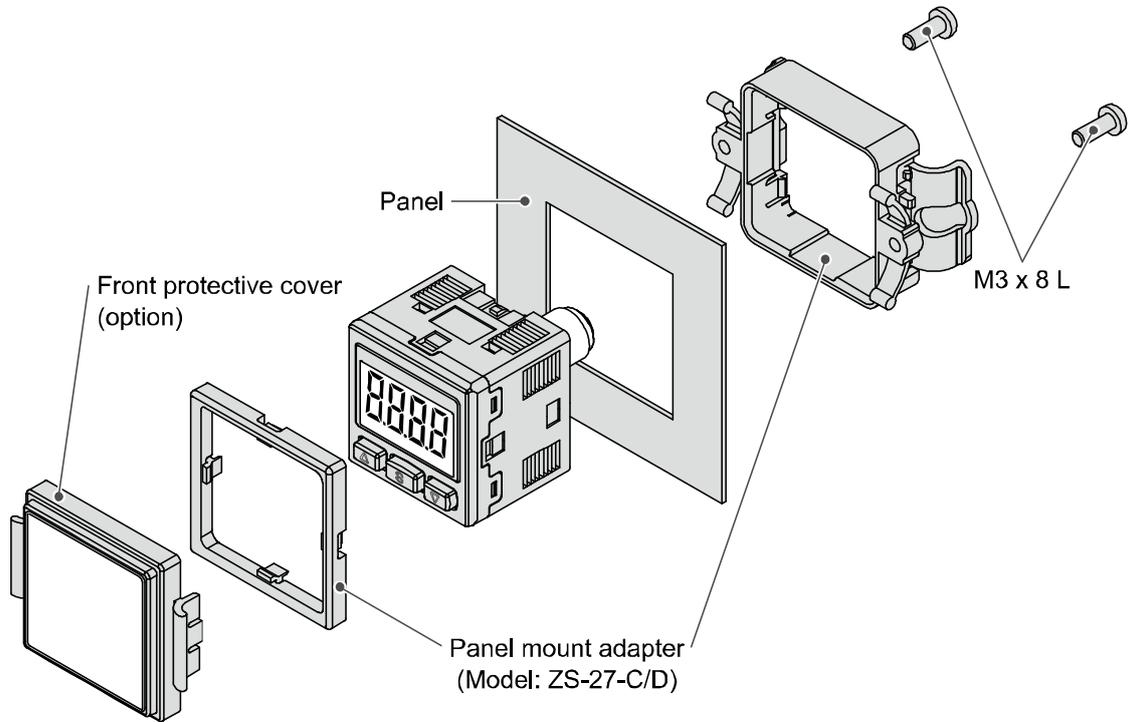
\*: The panel mount adapter can be rotated by 90 degrees for mounting.
