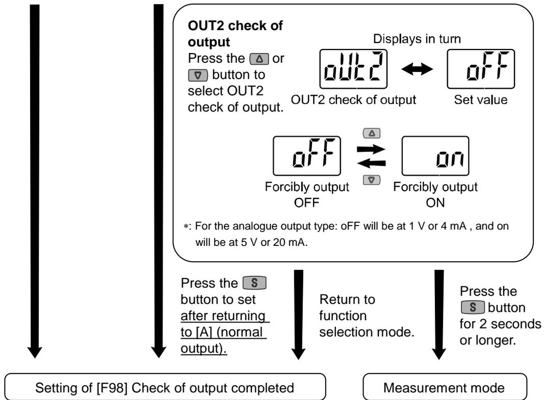
\*: If the button is pressed for 2 seconds or longer, the mode is returned to measurement mode regardless of the current mode.
