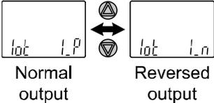
Press the SET button to set. ↓ Move on to pressure setting.
