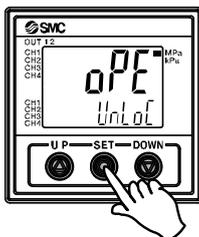
Press the UP and DOWN buttons simultaneously for 5 second or longer.
