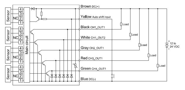
PSE201A-(M)□: PNP open collector 5 outputs + Auto-shift 1 input
