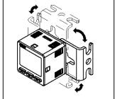
\*Bracket can be mounted on 4 sides.
