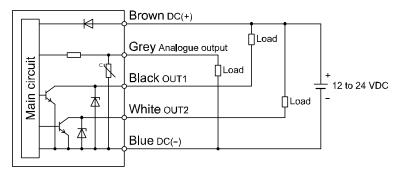
PNP (2 outputs) + analogue voltage output setting PNP (2 outputs) + analogue current output setting
