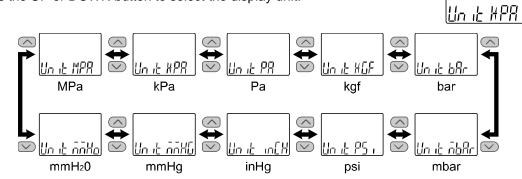
\*: The unit that can be displayed is different depending on the pressure range. (Refer to page 30) (kPa/MPa/Pa can still be selected if the product does not have the units selection function.)
