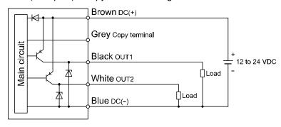
NPN (2 outputs) + analogue voltage output setting NPN (2 outputs) + analogue current output setting
