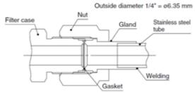
Weld the gland and piping when the fitting is used. At the time of welding, supply inert gas such as Nitrogen to the piping to prevent the formation of an oxide film. Also, remove the oxide film on the external surface through electrolytic polishing or acid cleaning. After tightening the nut by hand, add another 1/8 turn with a wrench to seal the fitting. Use the following parts for piping and fittings.
