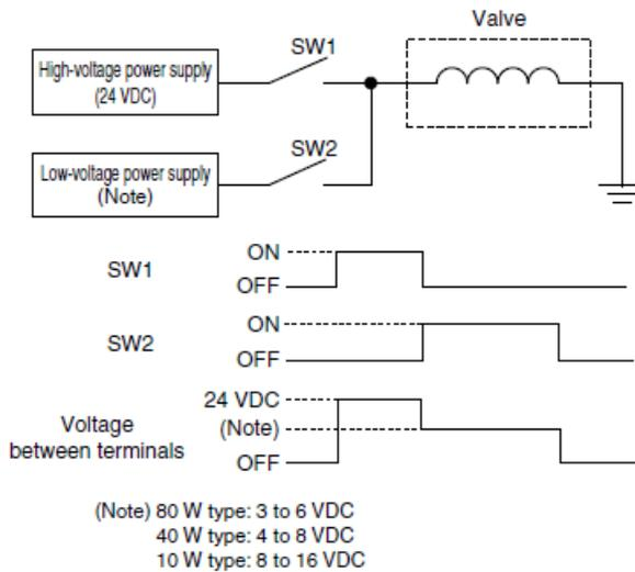
2. High speed switching control of high voltage by PWM control
