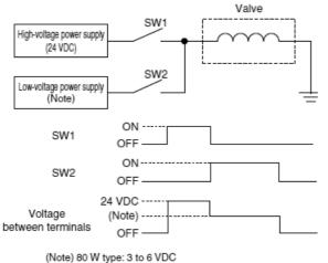
(Note) 80 W type: 3 to 6 VDC 40 W type: 4 to 8 VDC 10 W type: 8 to 16 VDC
