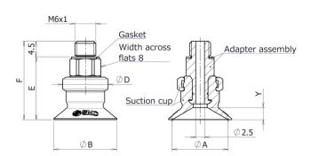
Model: ZPG\*C\*-7A-X2 (Suction cup form: Flat type with ribs)
