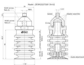
Note1) "D" and (st) indicate the reference value during gripping at vacuum pressure: -85[kPa].
