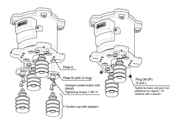
(1) Disassemble the suction cups with adapter
