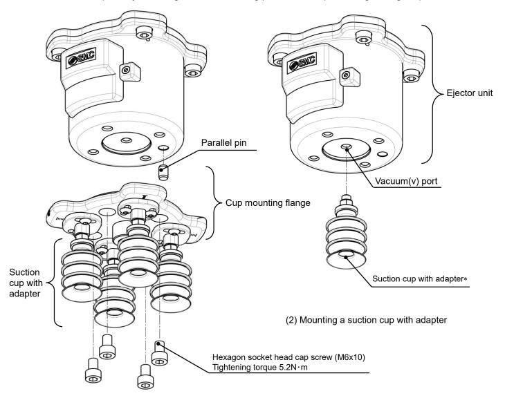
(1) Disassemble the cup mounting flange
