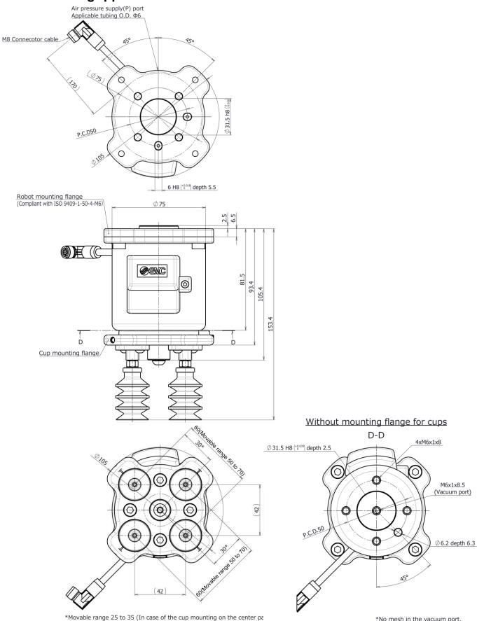
The suction cup diameter is necessary to be selected suitable for the cup piccn, because the cups may interfere each other depending on the diameter.
