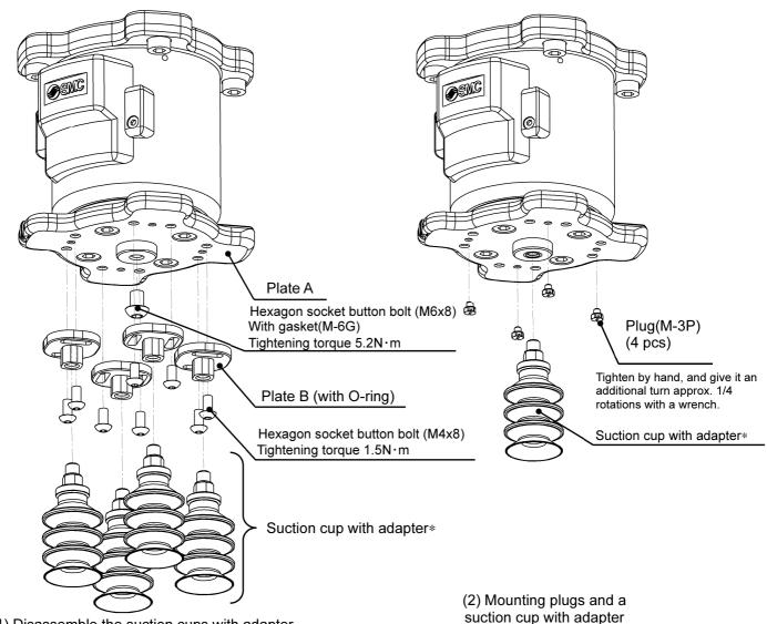
(1) Disassemble the suction cups with adapter
