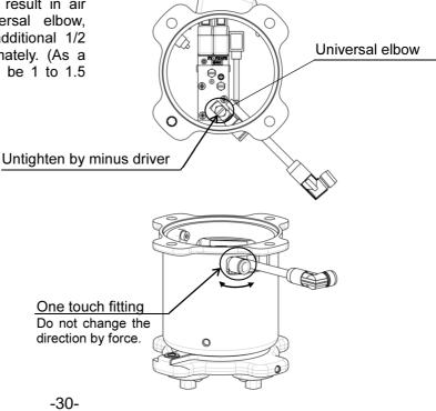
8) Adjust the length of air tube following by the movement of the robot arm to avoid adding tension the tube.
