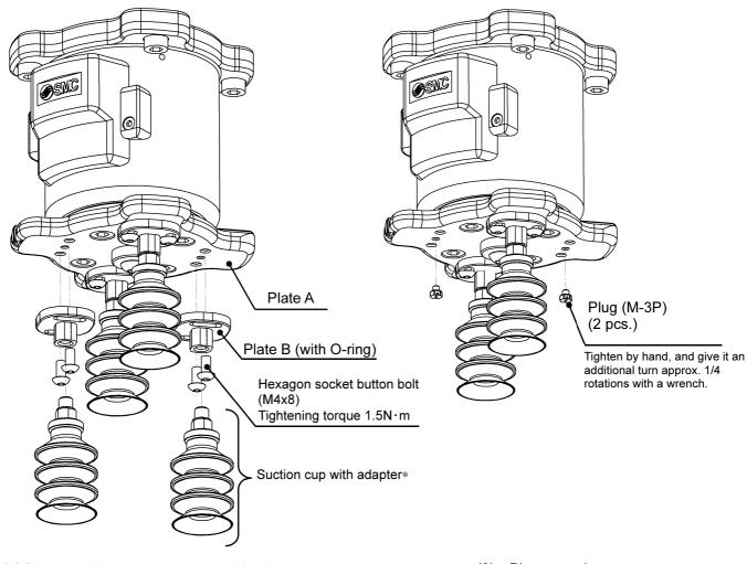
(1) Disassemble the suction cups with adapter
