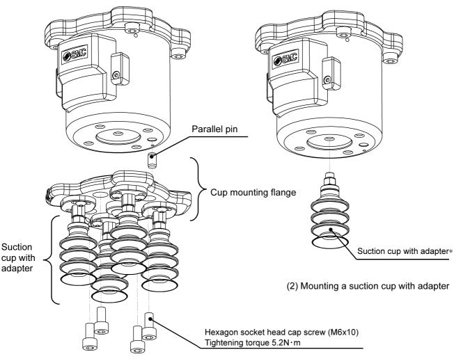
(1) Disassemble the cup mounting flange
