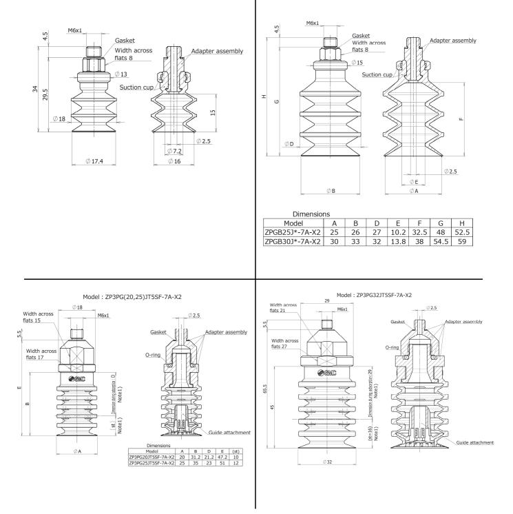
Note1) "D" and (st) indicate the reference value during adsorption at vacuum pressure: -85[kPa].
