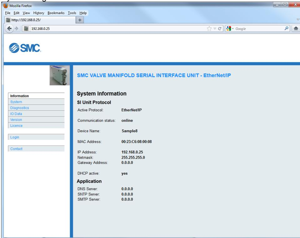
The screenshot shows a Mozilla Firefox browser window with the address bar set to `http://192.168.0.25/`. The page title is "SMC VALVE MANIFOLD SERIAL INTERFACE UNIT - EtherNet/IP". On the left, there is a navigation menu with options: Information, System, Diagnostics, IO Data, Version, Licence, Login, and Contact. The main content area displays "System Information" under the "SI Unit Protocol" section. The information includes:
