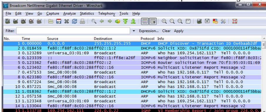
In this example the IP address of the SMC module is 192.168.0.11 as shown above at line 7.
