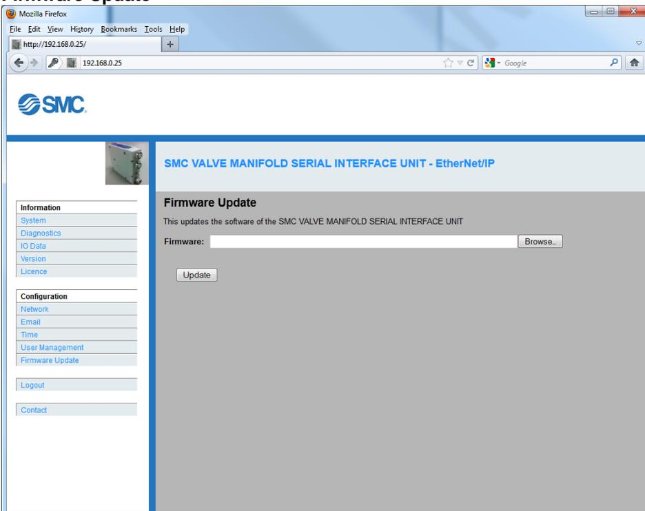
If a firmware update is required contact SMC for assistance. To download the new firmware, select the "Firmware Update" under "Configuration" tab. Browse and select the new firmware and click on Update.
