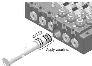
Apply vaseline (commercially available) on the O-ring surface, and insert straight. (Note the direction shown on the label.)
