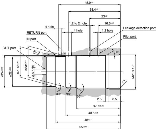
\* Recommended surface roughness of inner surface where the valve is inserted is Rz6.3.
