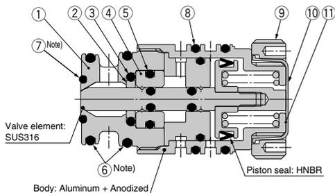
**Diaphragm / 2 liquid paint type VCC12D-00**
