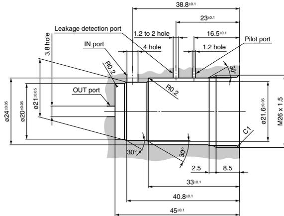
\* Recommended surface roughness of inner surface where the valve is inserted is Rz6.3.
