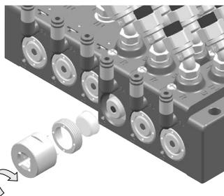
After mounting the indicator lamp cover, tighten the mounting nut to a tightening torque of 2.5 to 3.5 N-m of tightening torque.
