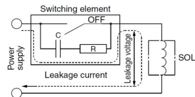
DC coil 2% or less of rated voltage
