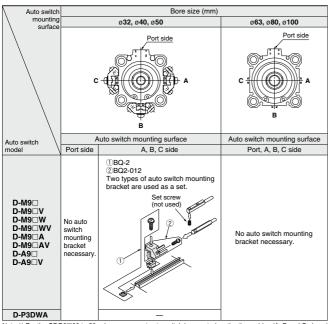
Note 1) For the CDQ2□32 to 50, when a compact auto switch is mounted on the three sides (A, B and C above) other than the port side of bore sizes a32 to a50, the auto switch mounting brackets above are required. Order them separately from cylinders. (It is the same as when mounting compact cylinders with an auto switch mounting rail, but not with a compact auto switch installation groove for the CDQ2□63 to 100.) Example
