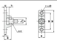
Material: Chromium molybdenum steel (Nickel plating)
