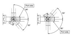
Push the one-touch connecting pin into the cylinder body (Double clevis) until it clicks and is firmly fastened.
