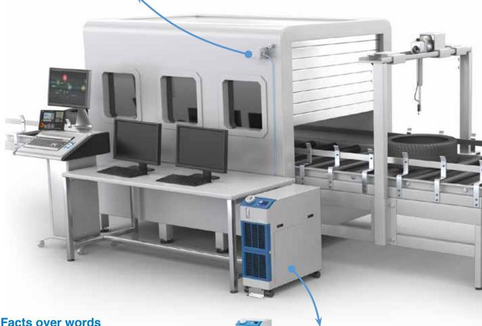
The compressed air of a balance testing operation was proven to contain water drops and oil mist, leading to inadequate air quality. By installing a combination of SMC's water separator, filter and mist separator, the air flow fulfilled the appropriate quality standards that the application required, leading to reliable operation.
