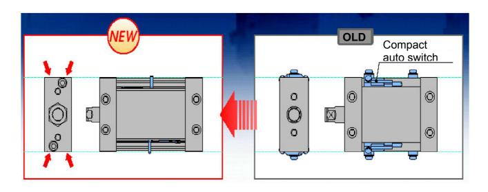
2. Adoption of the switch holding bracket. Reduction in man-hour required for mounting auto switches.
