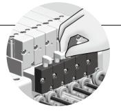
Solenoid valves can be replaced individually without shutting off the main pressure! Note)
