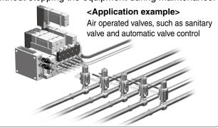
Note) This product is only for internal pilot specifications, as the external pilot air cannot be shut off.
